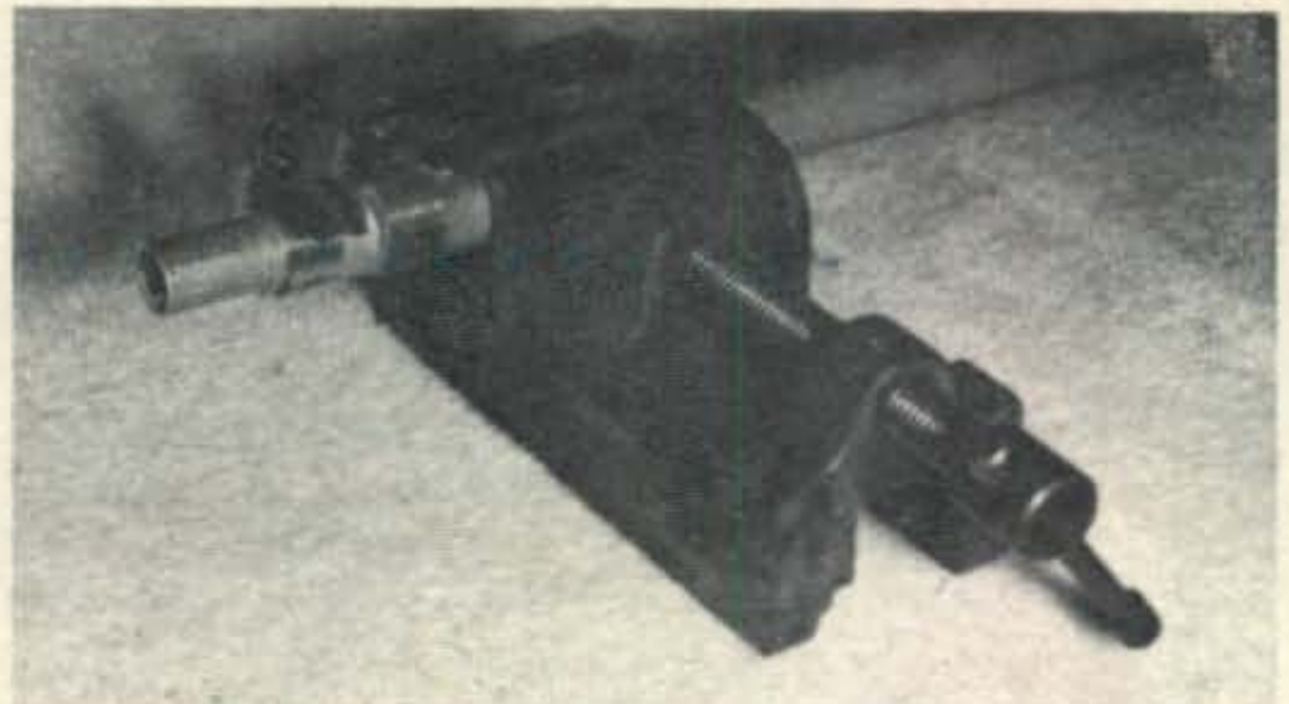
Fig. 3—Clamps are placed in position and tightened just enough to prevent their slipping off but not enough to close the slots.
