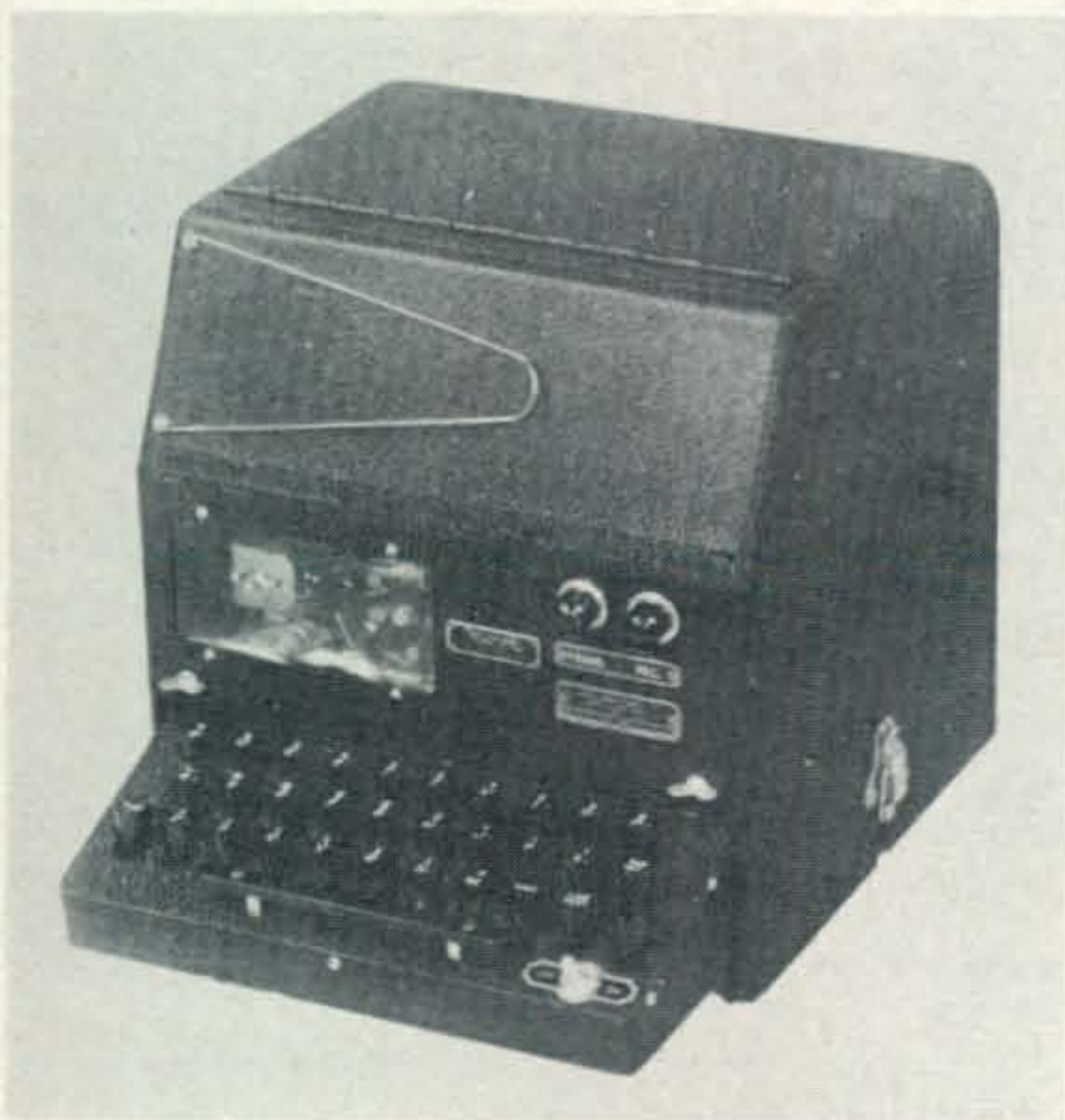
Fig. 1—The TT-30/AGA-1 Teletype Model #31 airborne tape printer, designed to print on standard 1/4 inch paper tape.
