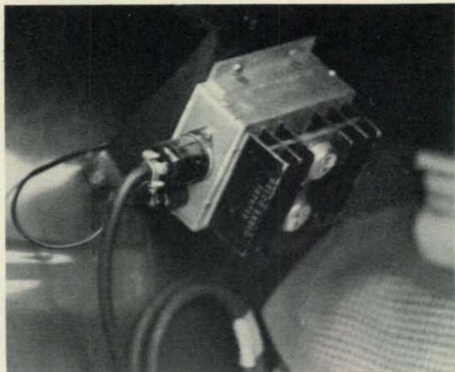
Fig. 4—View of the mobile supply mounted in the car shows location of the two switching transistors on the sink and of the power cable and fuse.
