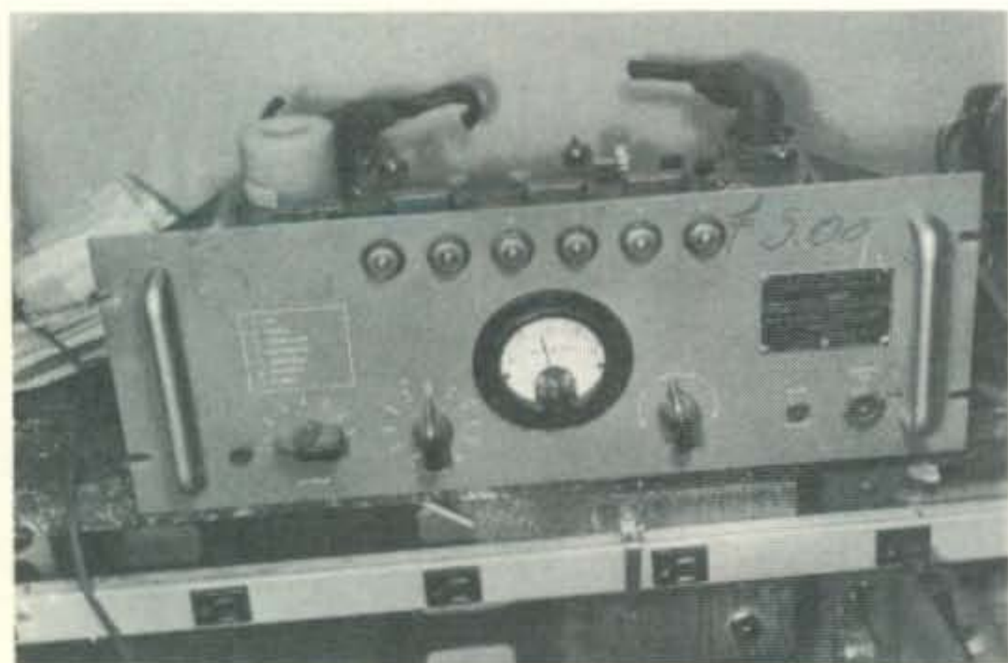
Fig. 1 — CV-81/FGC-5 transmitting code converter. This multiplex component is basically a serial-to-parallel converter which fed signals to the following stages of the multiplex transmitter.
