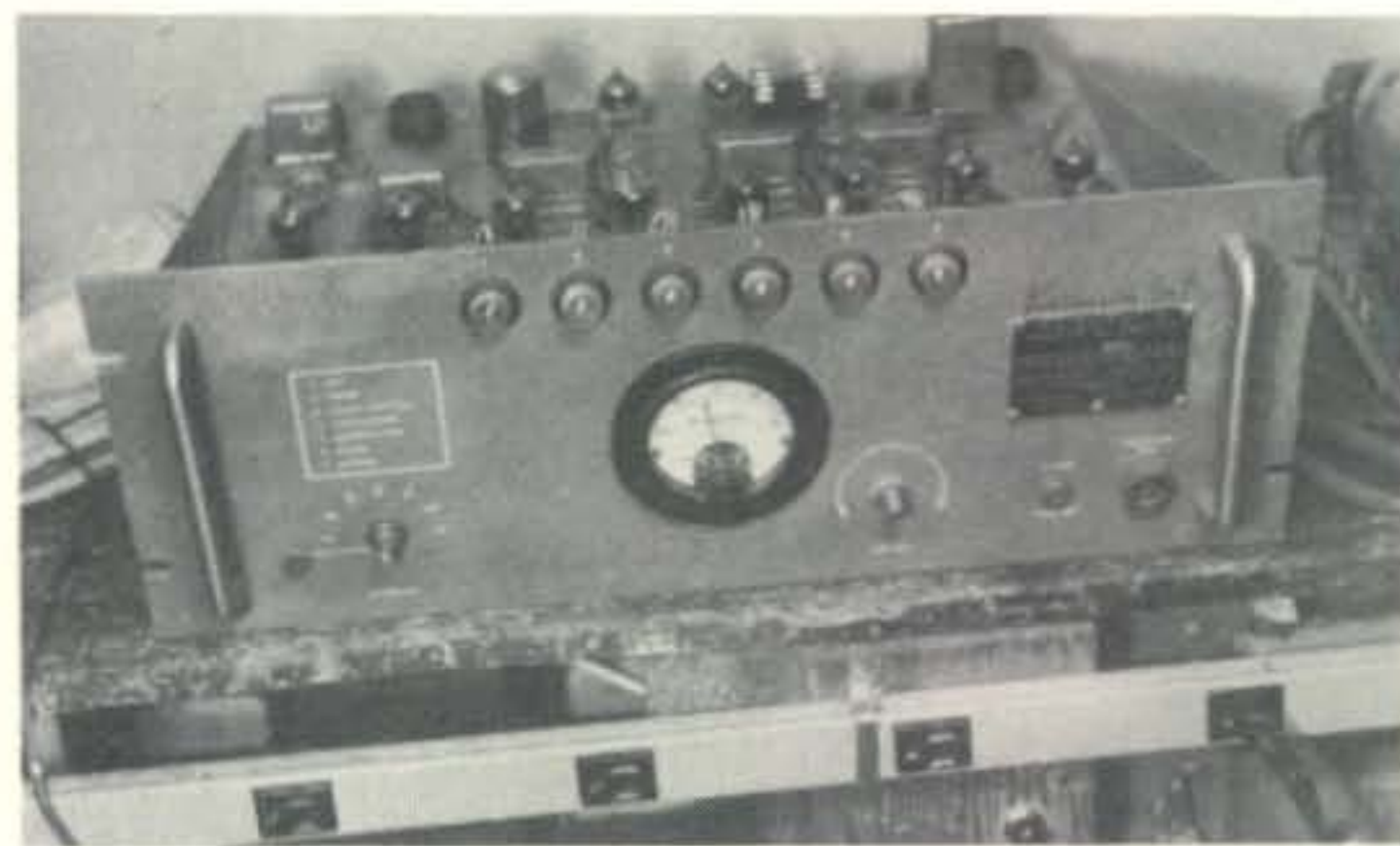
Fig. 2—CV-94/FGC-5 receiving code converter. A parallel to serial converter, the CV-94 will put a parallel output signal back into shape to be used by a Teletype printer.
