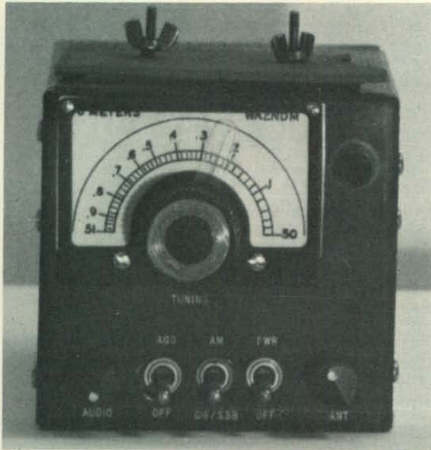
Front view of the 6 meter receiver. The controls are, from left to right, A. F. Gain, A.G.C. On/Off, AM-SSB, Pwr-Off and Ant.
