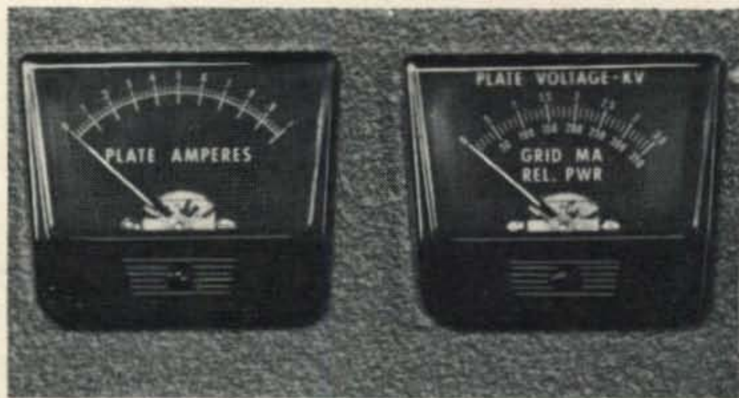
Complete monitoring facilities for fast, easy tune up. The left meter gives continuous monitoring of Ip . . . the right one can be switched to read Relative Power, Ep and Ig.
