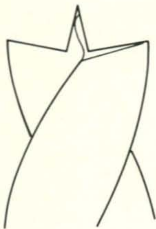
Fig. 2—The altered point is clearly shown in this view of the "sheet-metal" drill.
