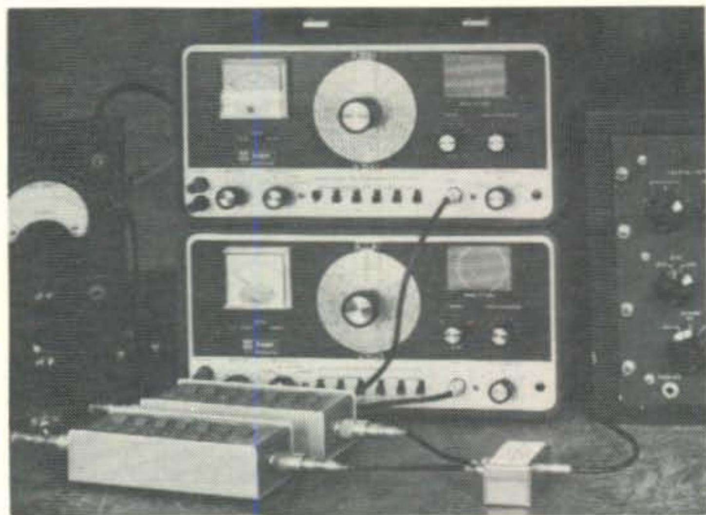
Test gear setup with Knight Kit KG-686 R.F. Signal Generators, Waters 371-1 Step Attenuators and composite combining network. The a.f. meter is on the left.
