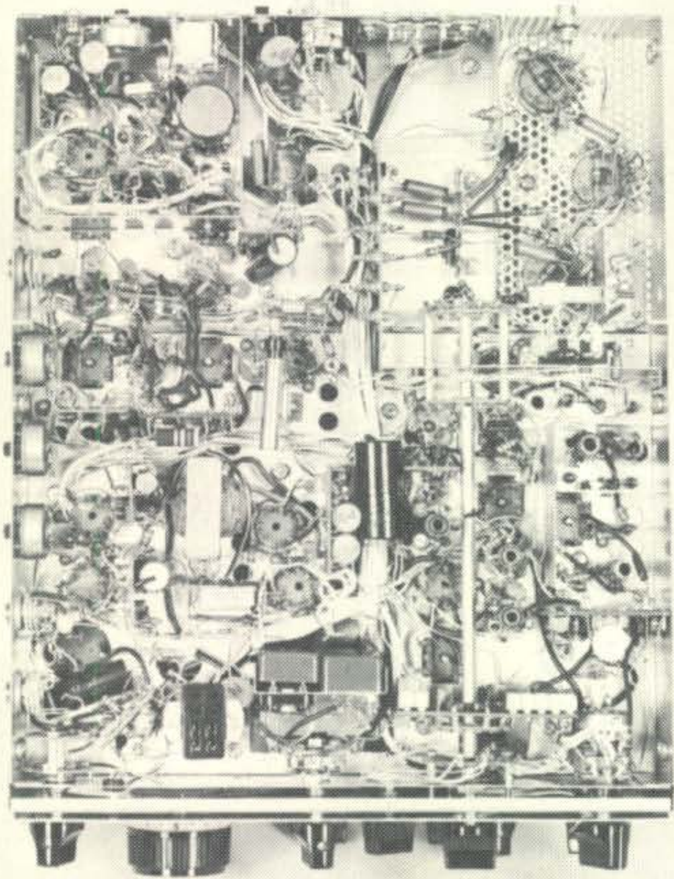
Bottom view of the TR-6. The solid-state sections are built on various small circuit boards mounted vertically below the chassis.
