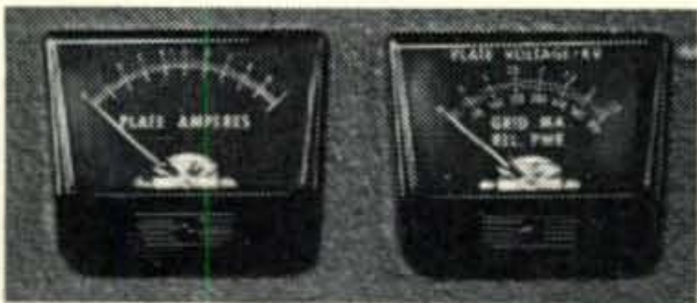
Continuous monitoring of Ip plus switch selected monitoring of Rel Pwr., Ep & Ig.
