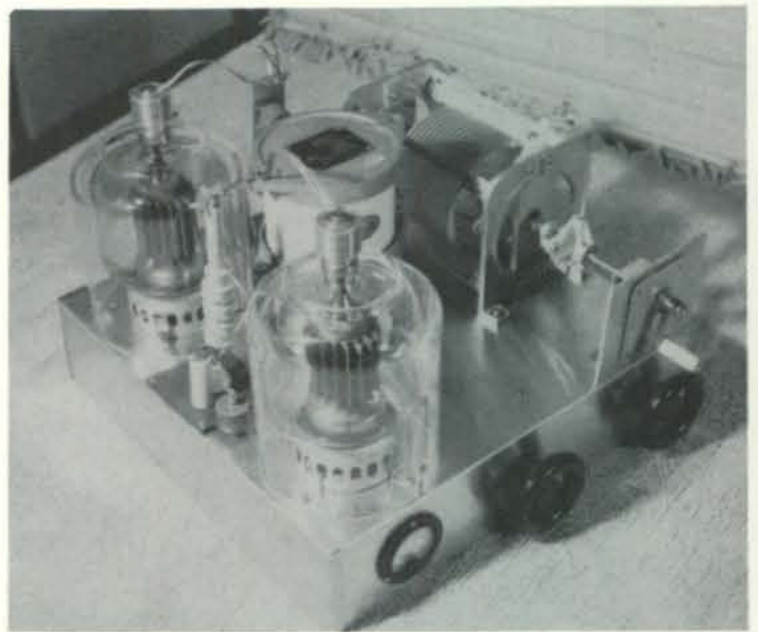
Top view of the linear showing the location of the major components.
