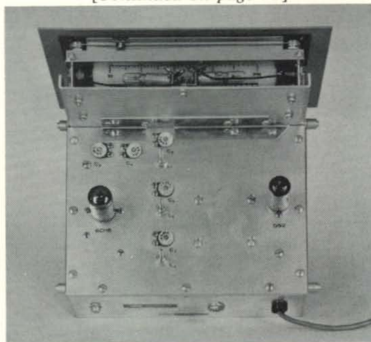
Top view of the HG-10B V.F.O. The adjusting screws for the inductor slugs and the trimmers are slightly to the left. Dial and drive mechanisms are between the vertical bracket and the panel. Other components are bottled up and well shielded within the chassis.
