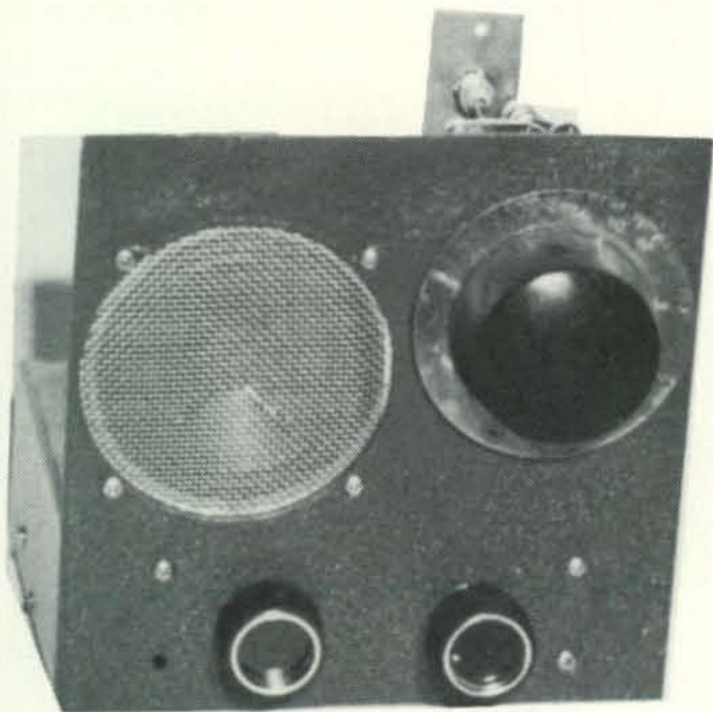
Front view of the two meter solid state v.h.f. regenerative receiver. This set is an ideal starting point for the Ham who wants to get his feet wet in solid state electronics.
