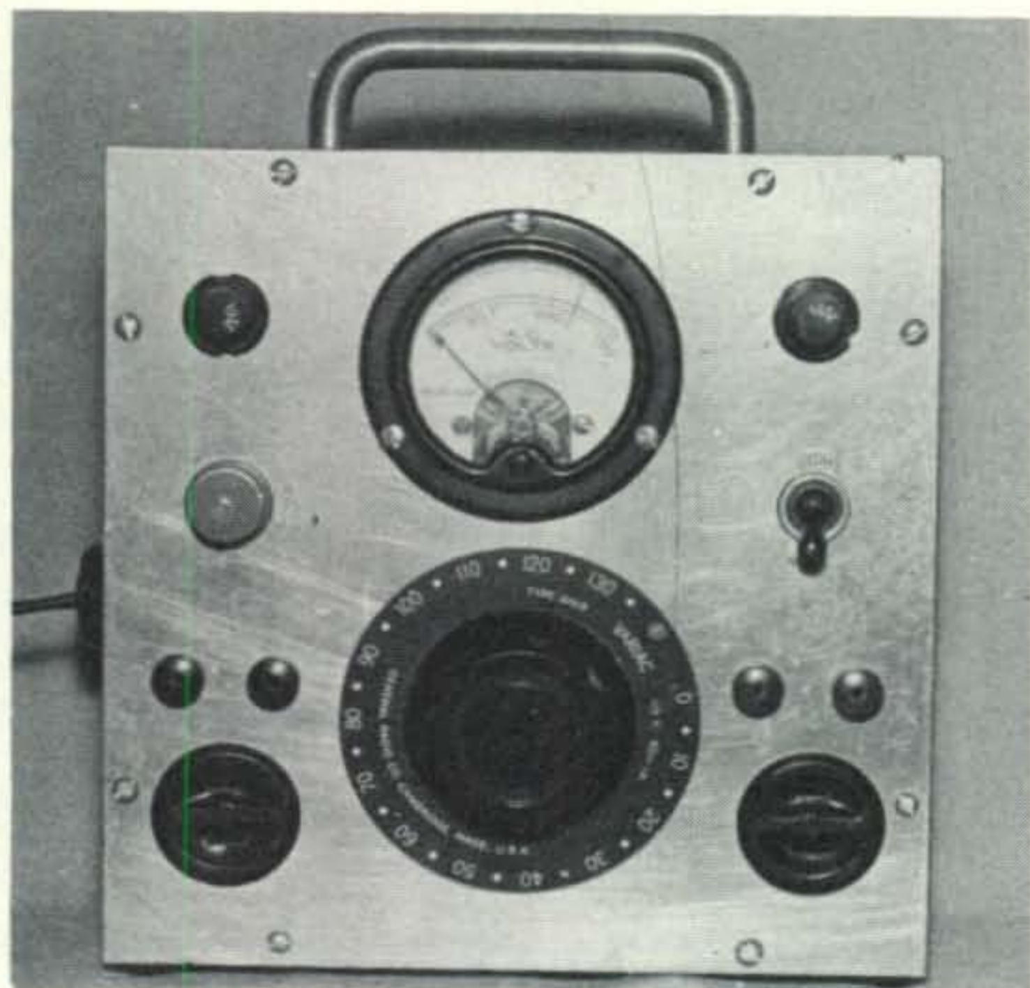
Front view of the variable a.c. supply. The jacks and switches are described in the text.
