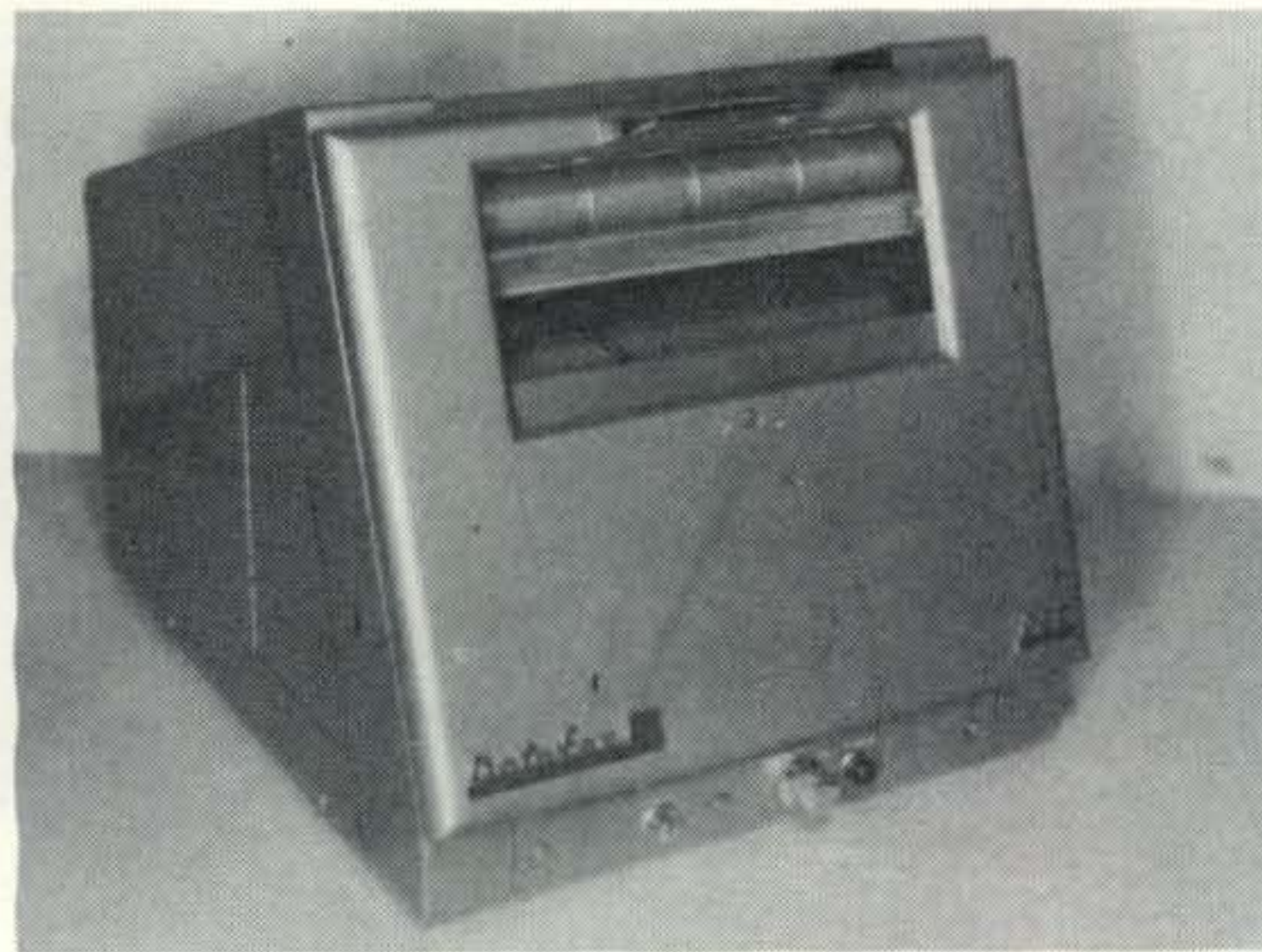
Fig. 3—The Datafax facsimile receiver and its associated transmitter.
