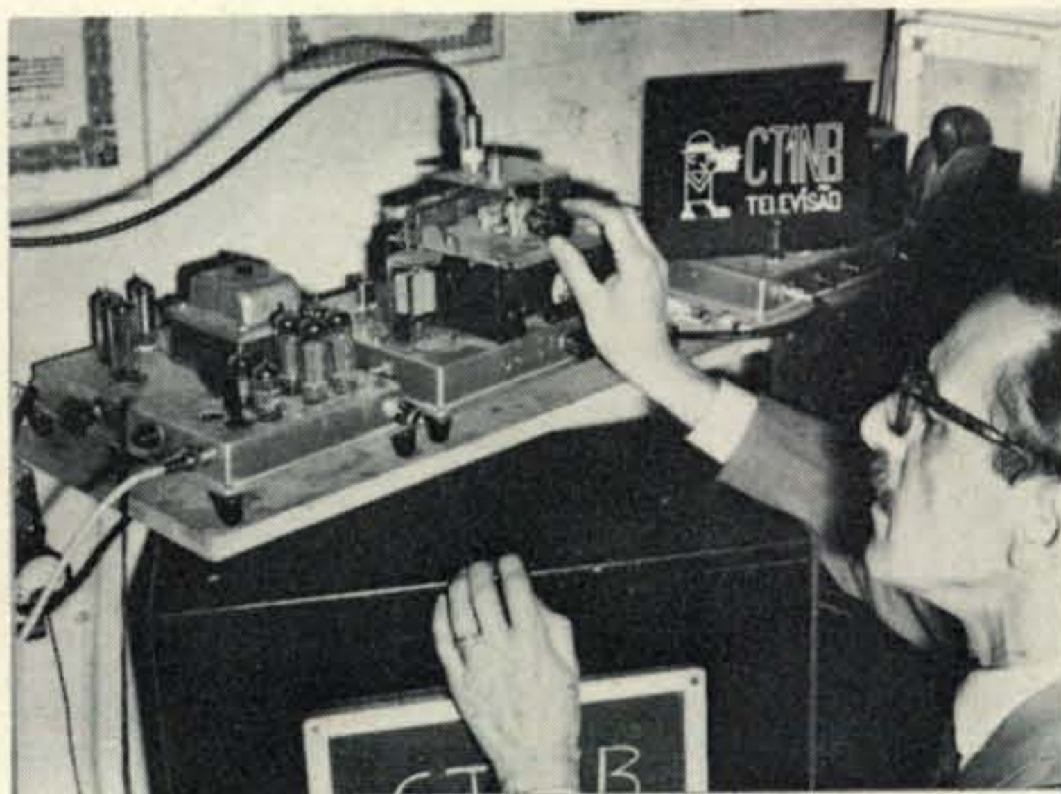
Roberto Charters de Azevedo, CT1NB-TV, tunes up the ATV transmitter. It is briefly described in the text.
