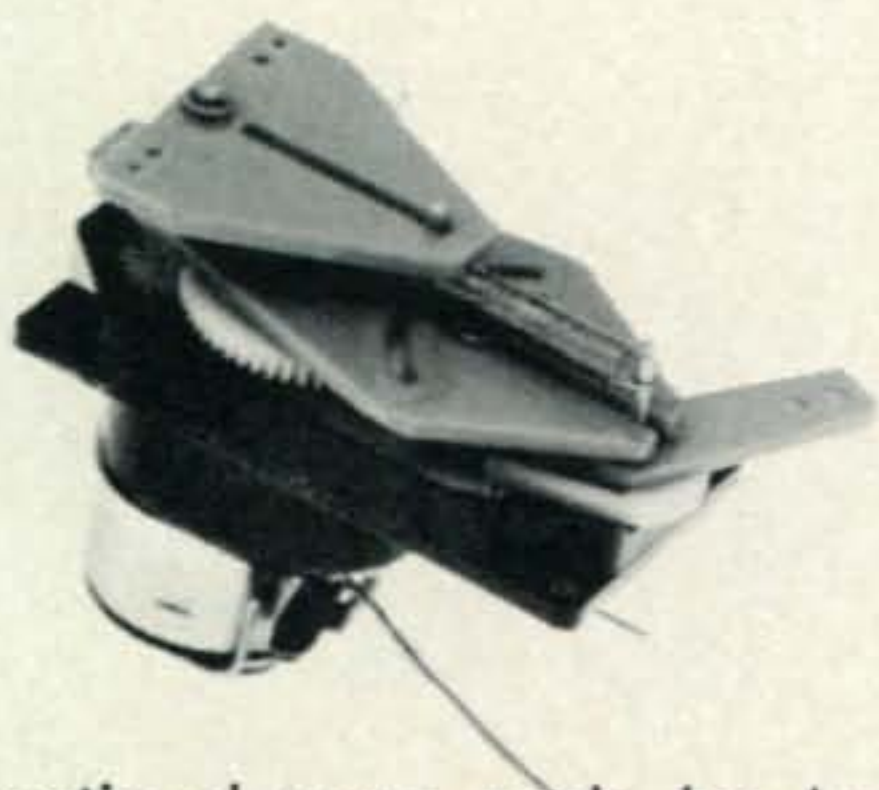
Pulse proportional servo made by Ace Radio Control. It allows rudder, elevator and throttle operation via pulse length rate changes. The small side arm is linked to throttle. Note the heavy centering spring.
