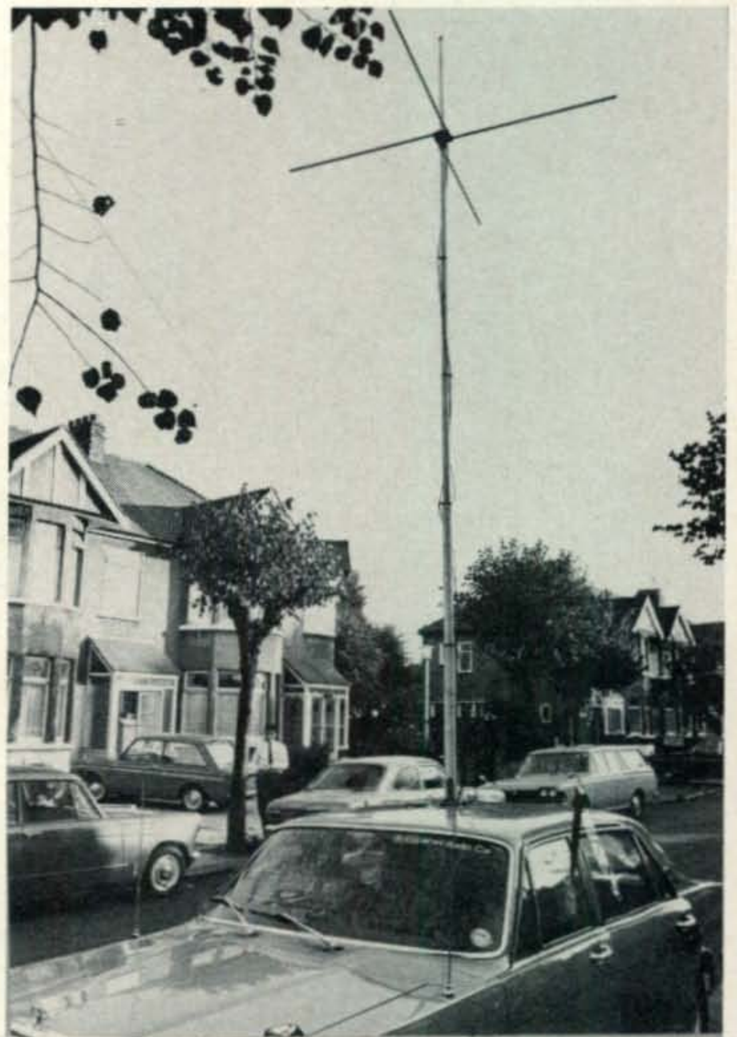
"This thing was bigger than any of us!"—the telescopic mobile antenna on the B.B.C. News Radio Car. A signal was transmitted direct back to the B.B.C. studio at Broadcasting House, 10 miles away.
