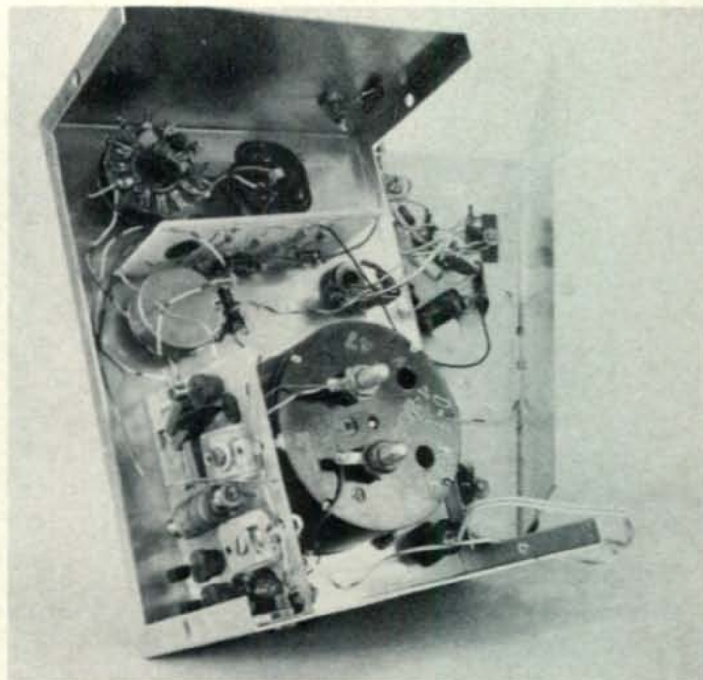
Interior view of the f.m. adapter. All components except those associated with the power supply and audio output stage are mounted in the front half of the box.
