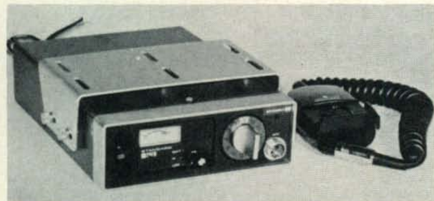
The Standard Communications Corp. model SR-C806MA 2-meter f.m. transceiver.
