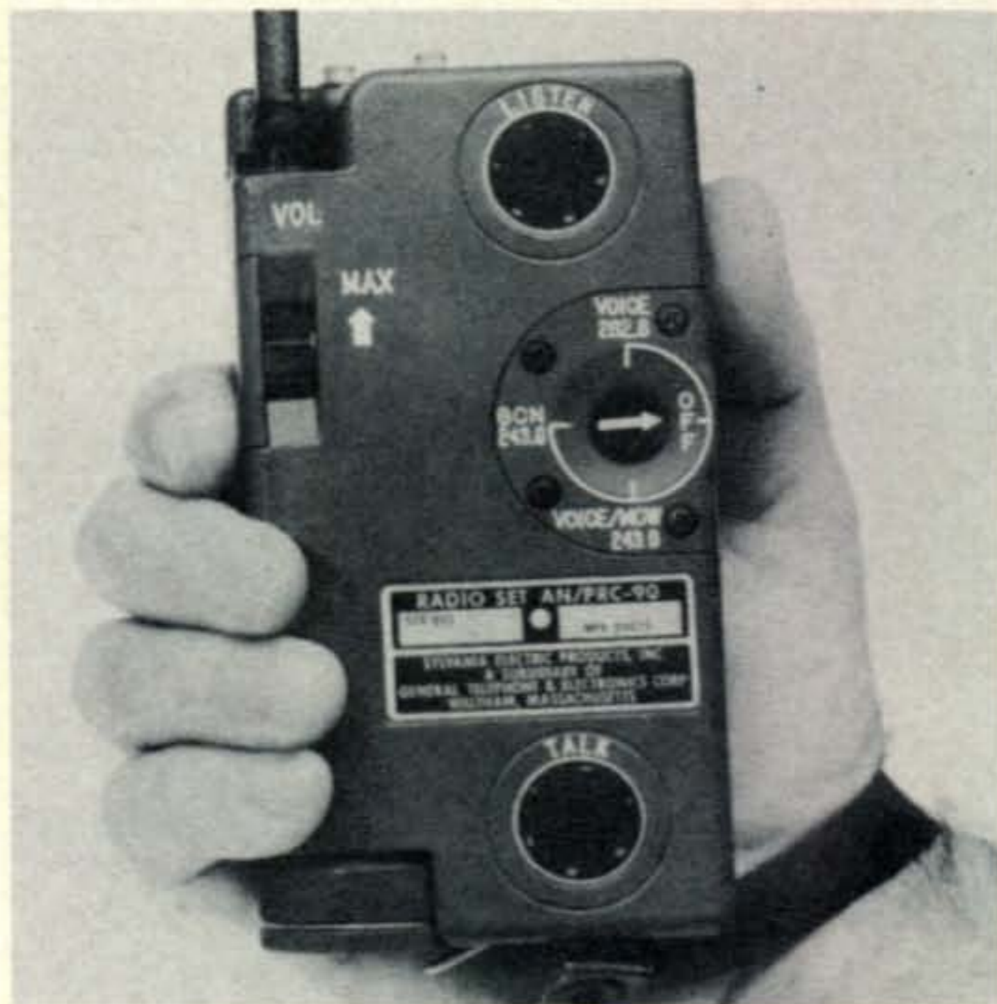
Fig. 4—This is the AN/PRC-90 u.h.f. dual transceiver. The same design is available in a high-frequency version. At 24 ounces, the PRC-90 costs the Army more than $20 an ounce.
