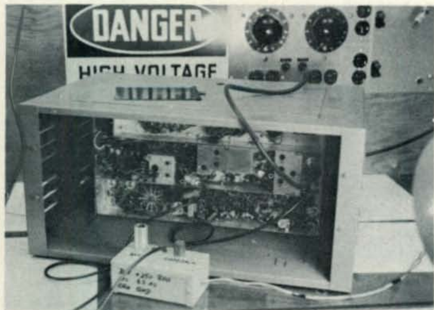
The simple Q-multiplier of fig. 2 is shown connected to a Motorola Station Monitor through a BNC connector mounted close to an i.f. amplifier.
