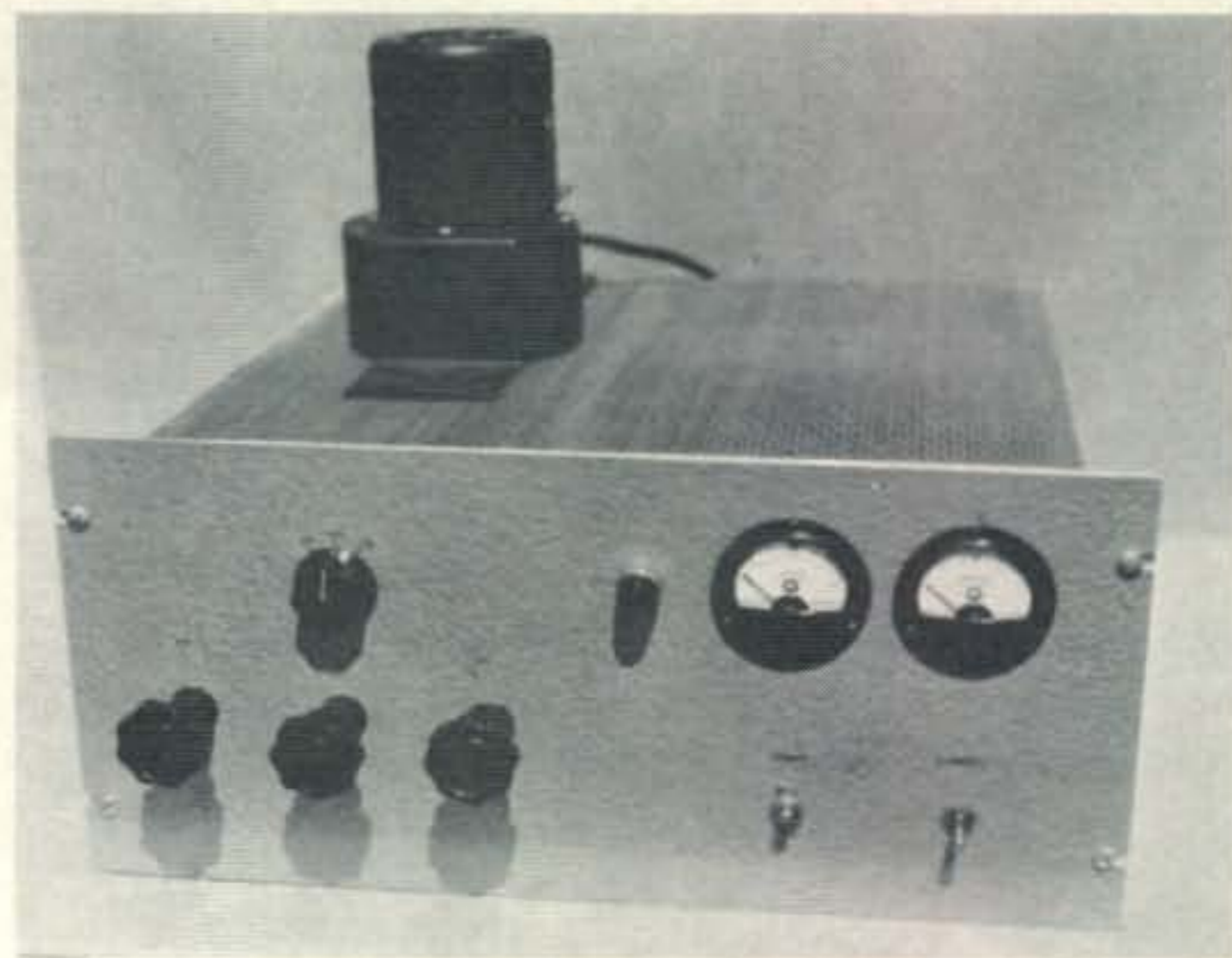
The Table-Top Maxi Linear is completely self-contained, with power supply, behind an 8 \frac{3}{4} " high standard rack panel. The obvious exception is the extra exhaust blower mounted above the 3CX1000A7 amplifier tube.
