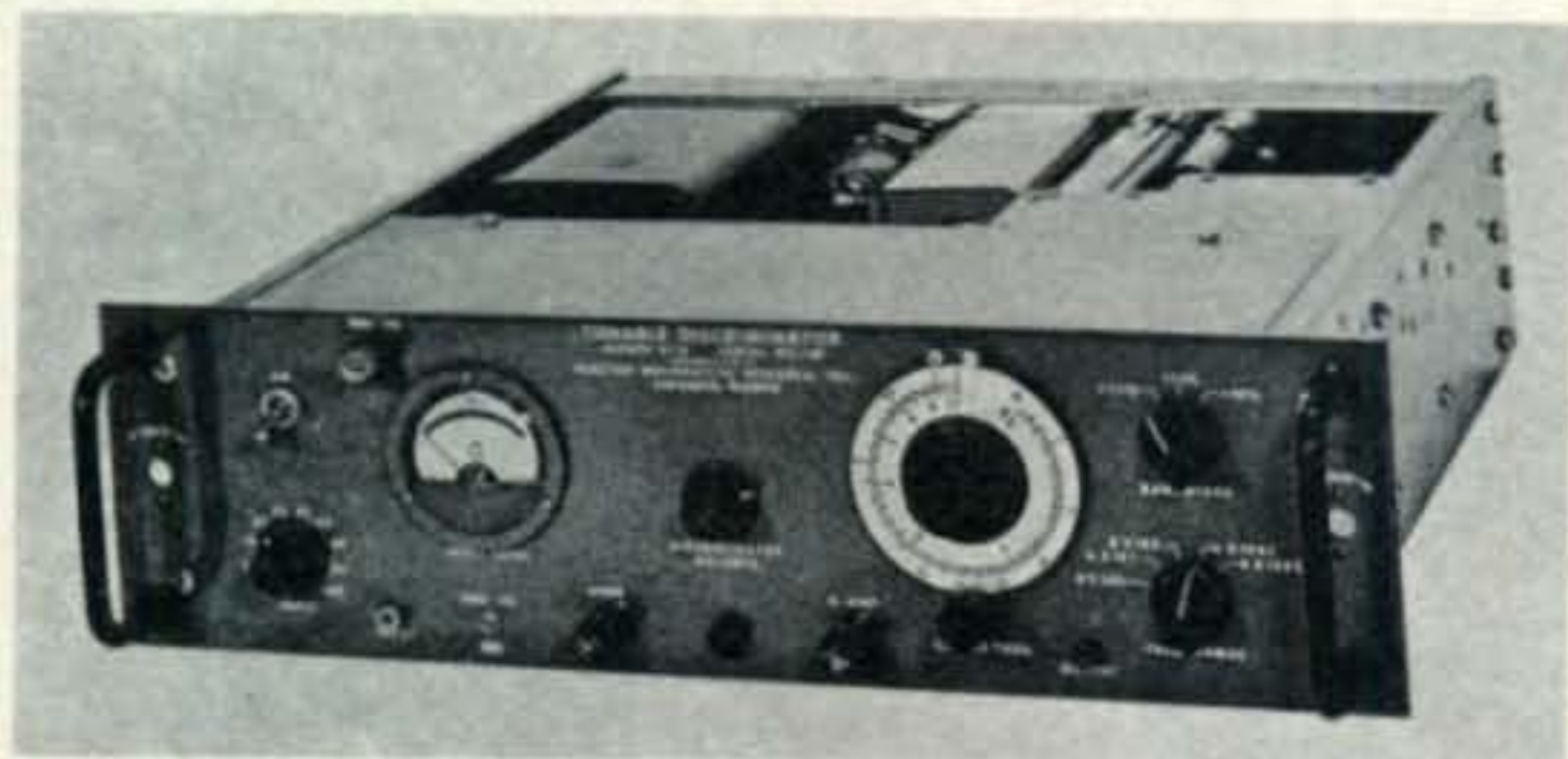
Fig. 1—Tunable audio discriminator, used in N.A.S.A. Telemetry reception, makes an excellent RTTY discriminator when coupled with other surplus gear and a simple loop keyer.
