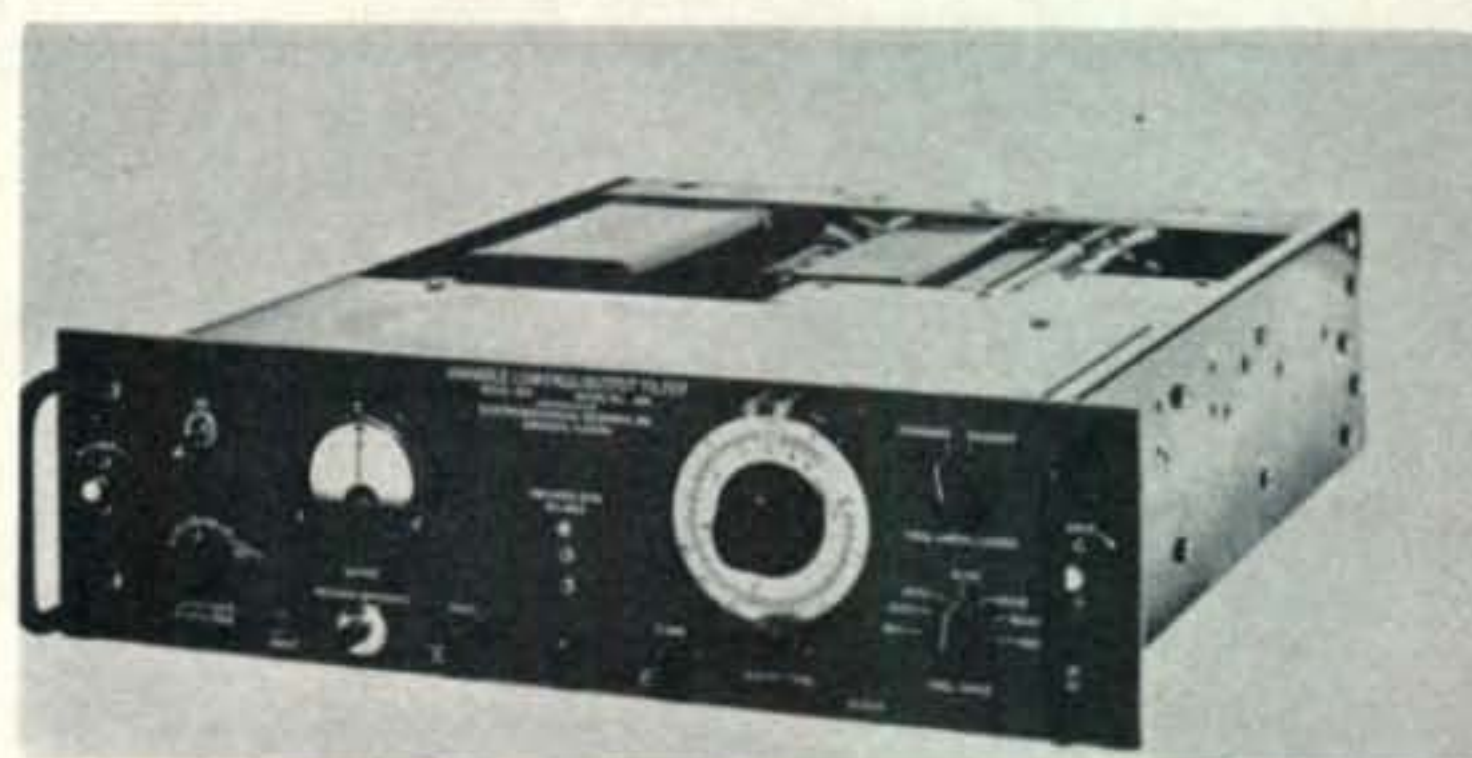
Fig. 2—Variable low-pass filter, following the tunable discriminator (fig. 1) makes a good amateur RTTY receiving setup.
