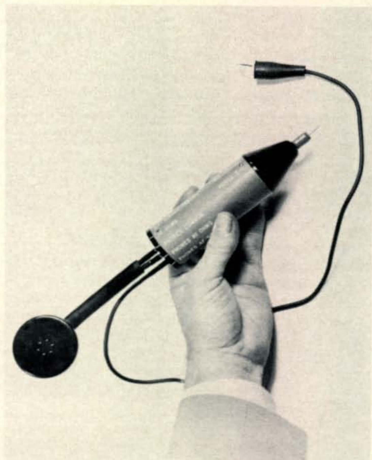
The LEL Dynamic Serviset Model E-C. The "common" test lead at the left is plugged into one of the phone-tip jacks provided for the various functions. The prefocused lamp is at the center of the ring of jacks. The neon lamp is behind the hole in the side of the barrel. The plug-in headphone is at the left.
