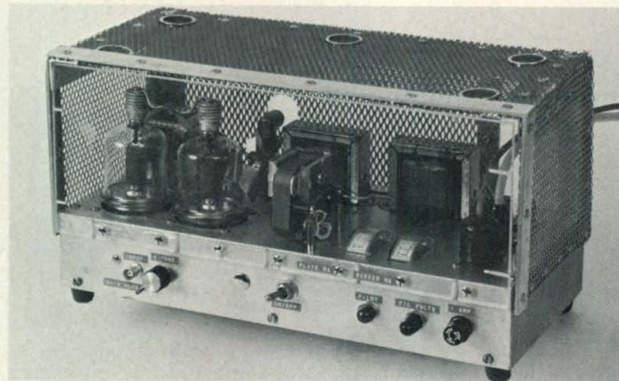
An overall view of the 500 watt linear in its case. Both PL-177WA tubes are mounted on conventional Johnson septar sockets without chimneys. A Barber-Colman transverse blower delivers 190 c.f.m. to cool the pentodes and blocking capacitor. (A 3" fan is shown here but was changed later to a 4" model.) The controls on the front are from left to right; grid input, grid tuning, power on-off, power indicator, filament indicator and filament fuse.
