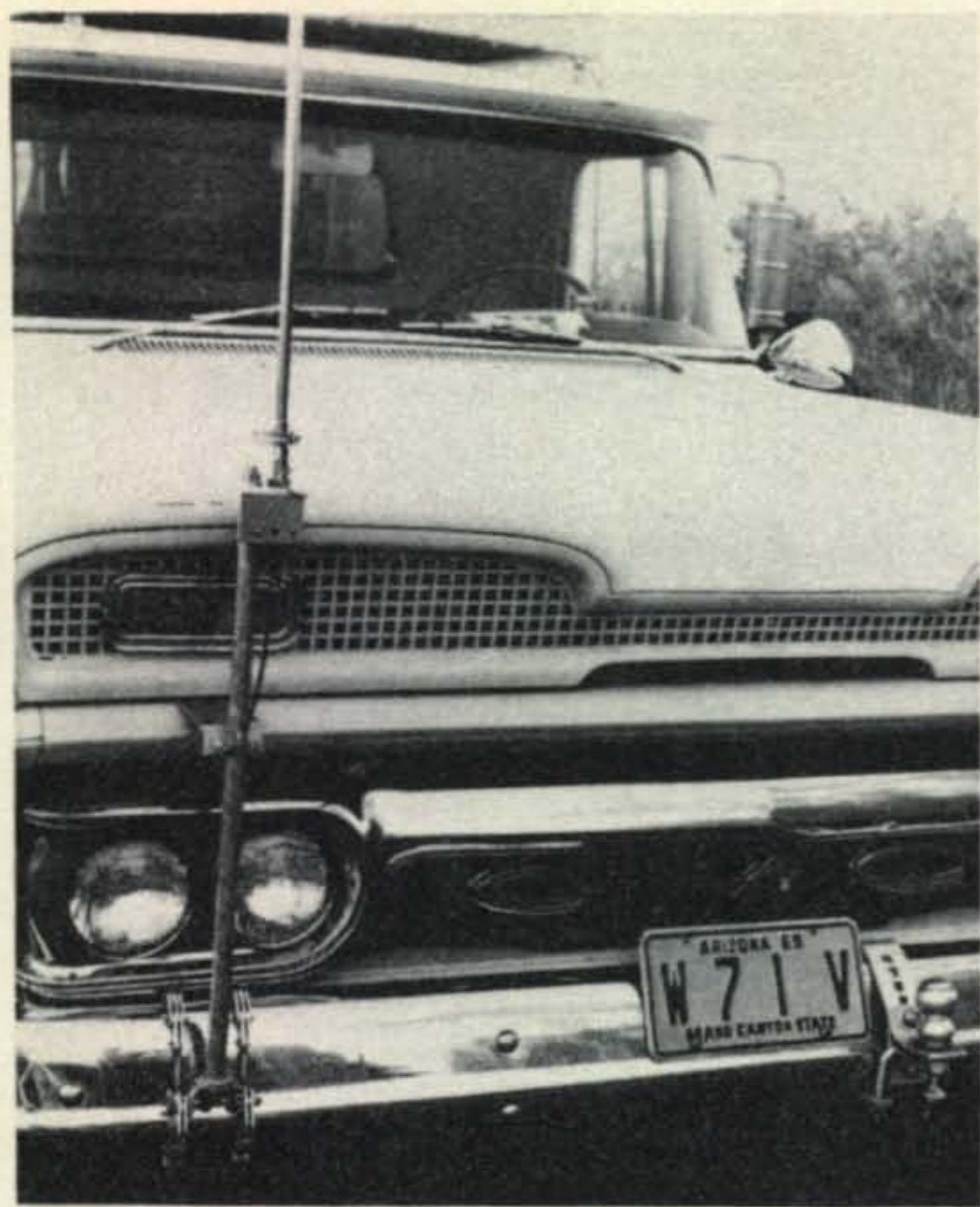
Front view of the camper truck showing the system used to elevate the whip antenna to a position even with the hood of the truck.
