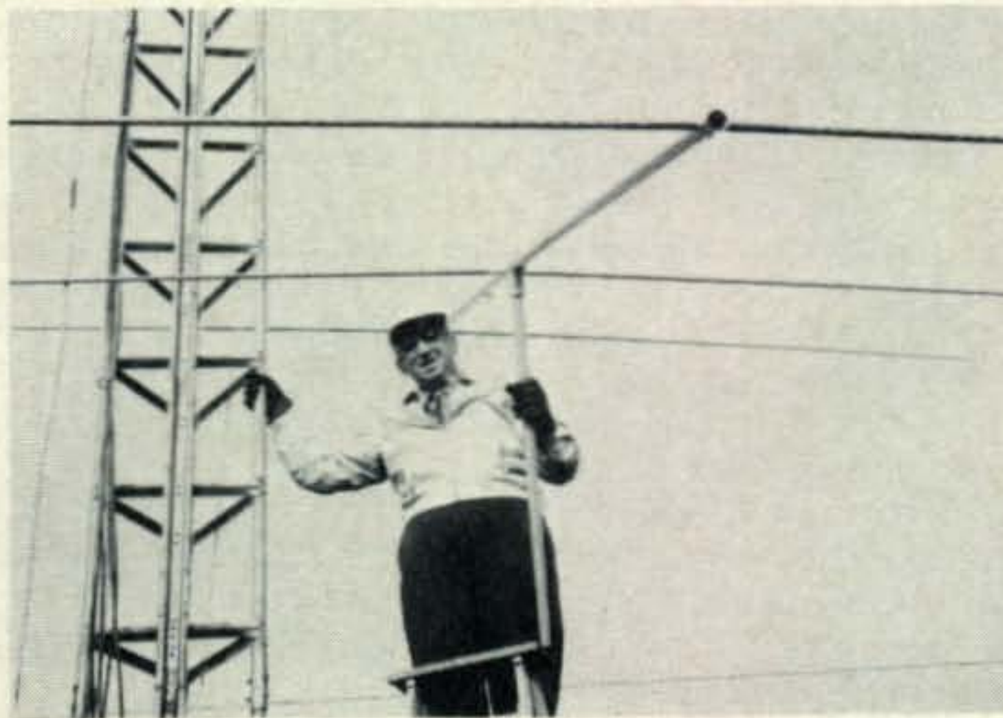
Kirk Chief Engineer "Doc" Self is shown holding a 3-element 20-meter beam—all of 19 lbs!
