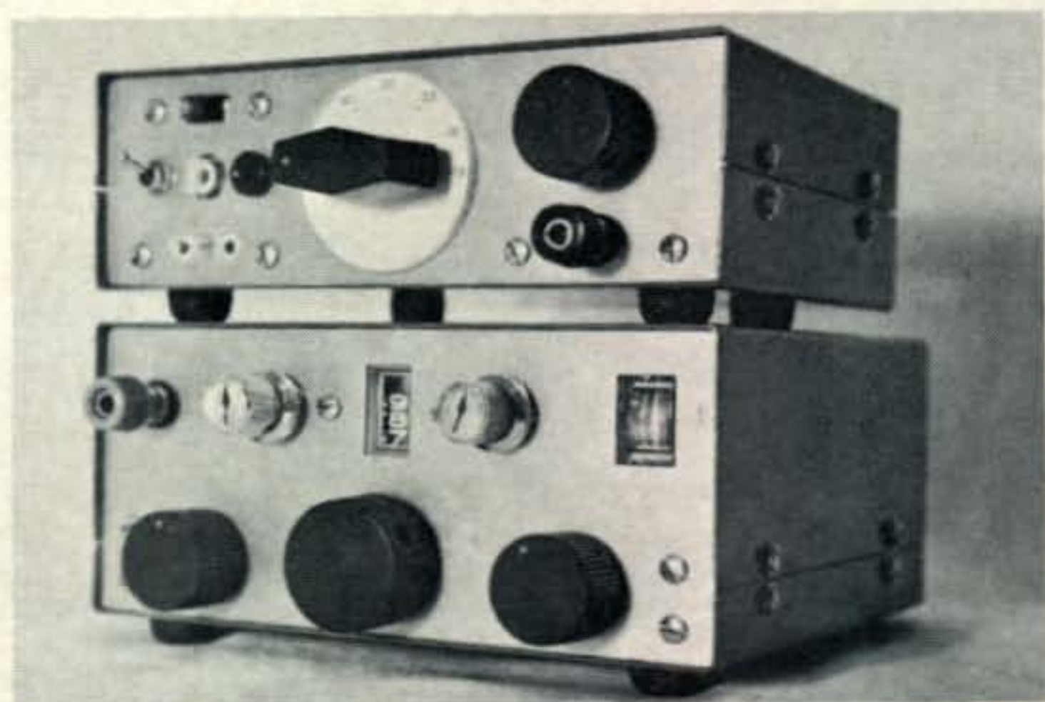
The converter is shown atop its companion receiver, the GP-32. Converter controls are (left to right): slide switch for calibrator above power on/off toggle switch, RCA jack for converter output, calibrator output jack, crystal socket (bottom left), bandswitch, antenna input (bottom right), antenna trimmer (top right). Bandswitch dial marking is in wavelength for shortwave BC bands.
