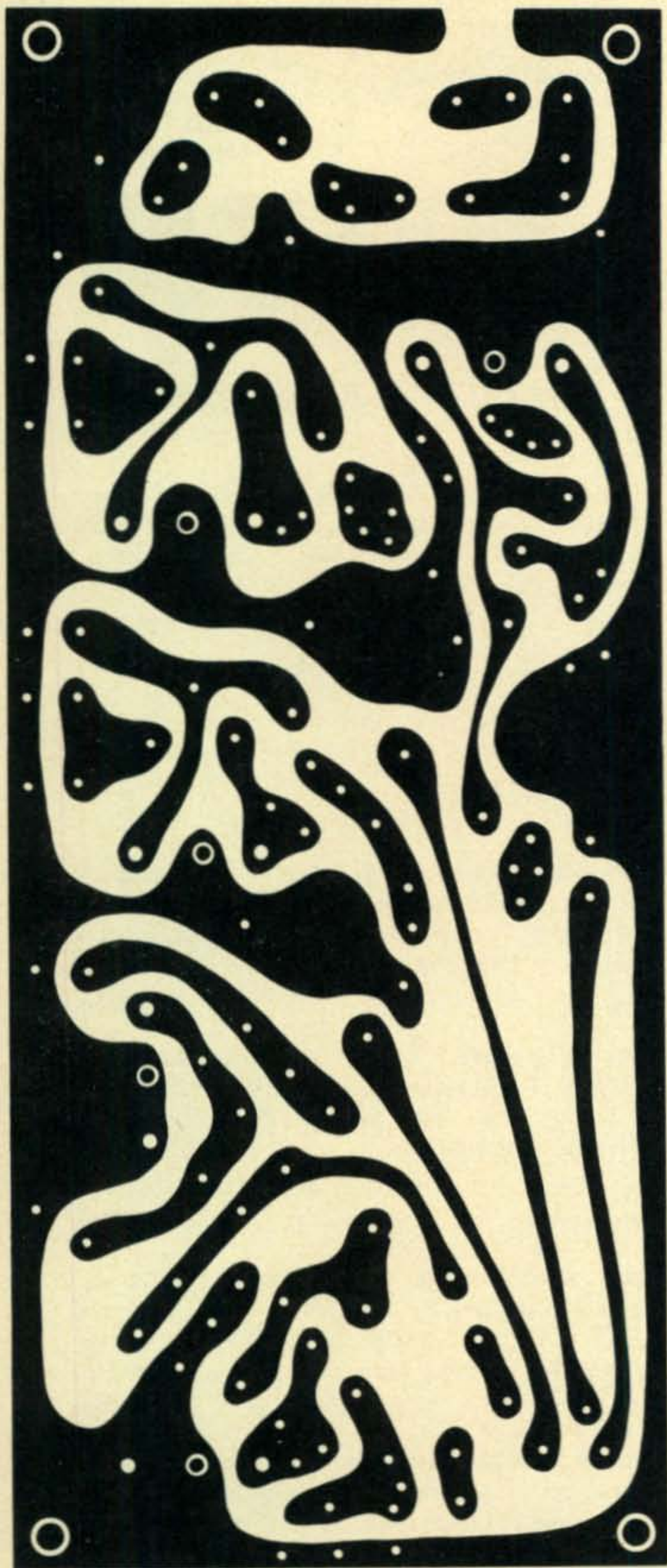
Fig. 2—Actual size circuit board layout for the s.w.r. bridge built-in signal source and parts layout for the circuit board. Component numbers shown correspond to those in fig. 1.
