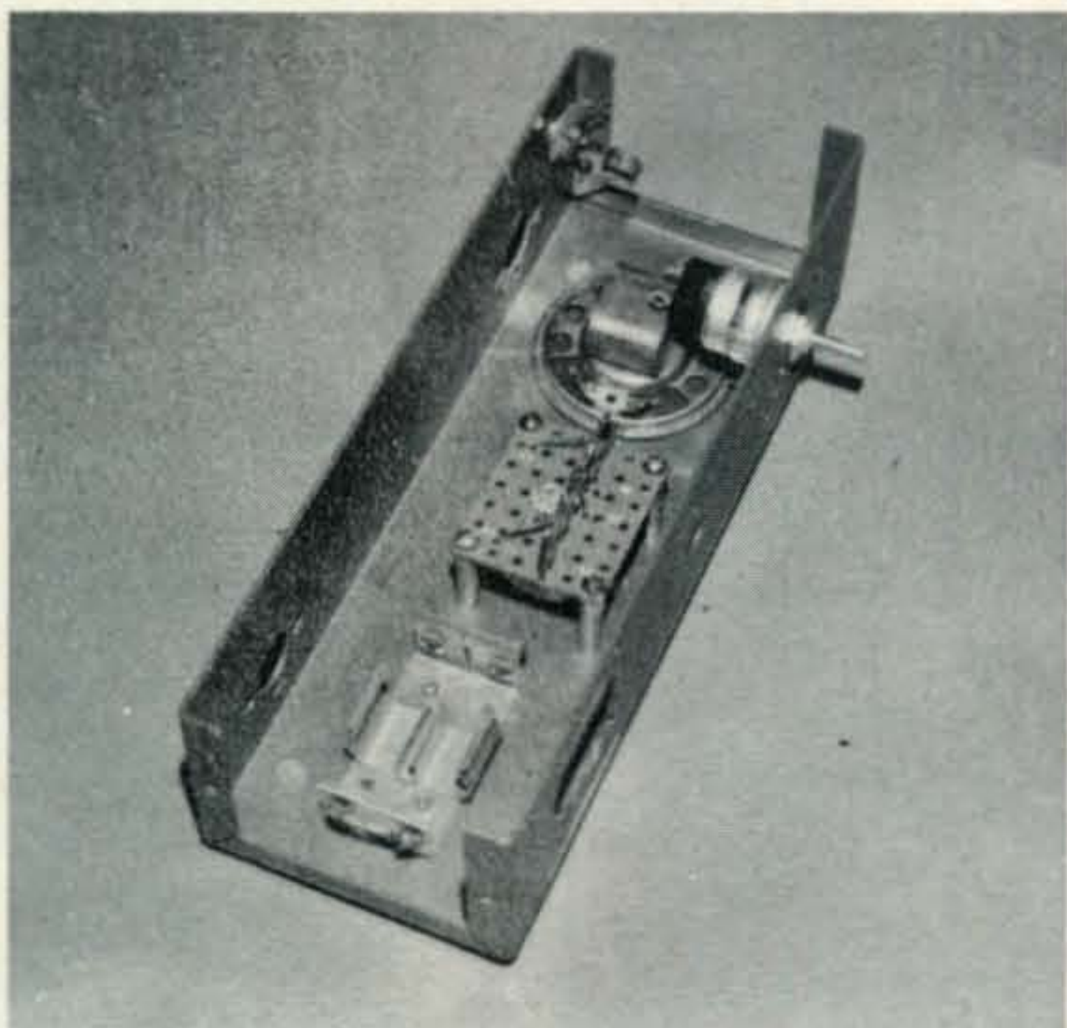
Side-Bridge components to be added are trial-fit inside the HW-15 s.w.r. bridge cabinet.
