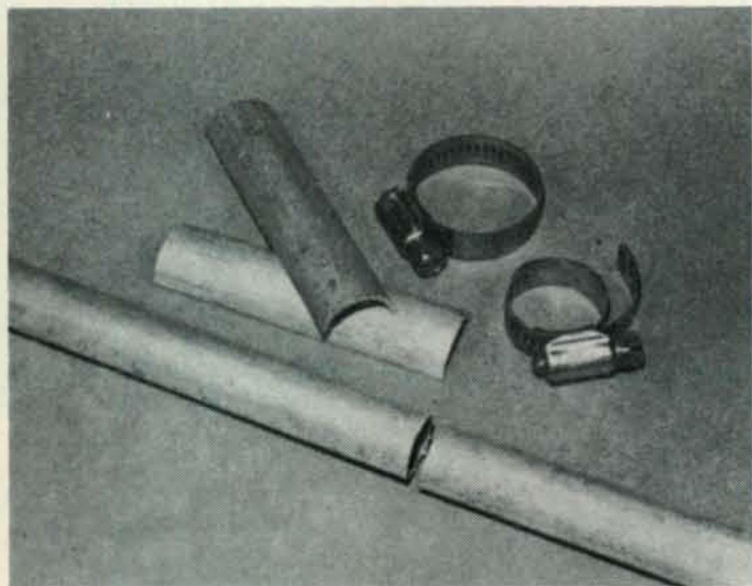
Use 6" half shells with two hose clamps to join lengths of tubing to achieve the needed 16' dimension.
