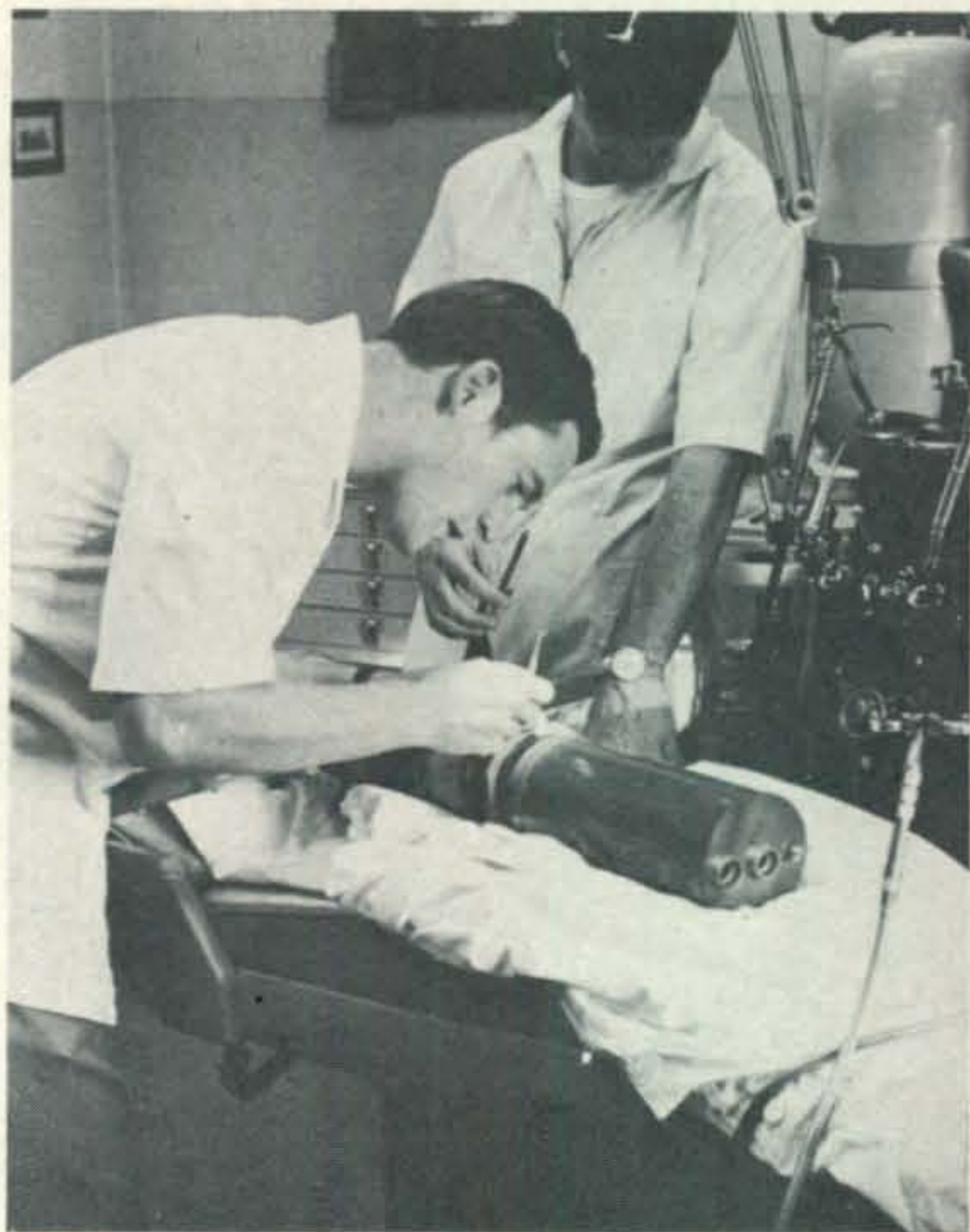
Lieutenant Reid J. Talcott III, DC, USNR, of NAVCOMMSTA Morocco Dental Department, applies amalgam to pitted area in high powered klystron. Dr. Talcott was assisted by DN Robert R. Pierce.
