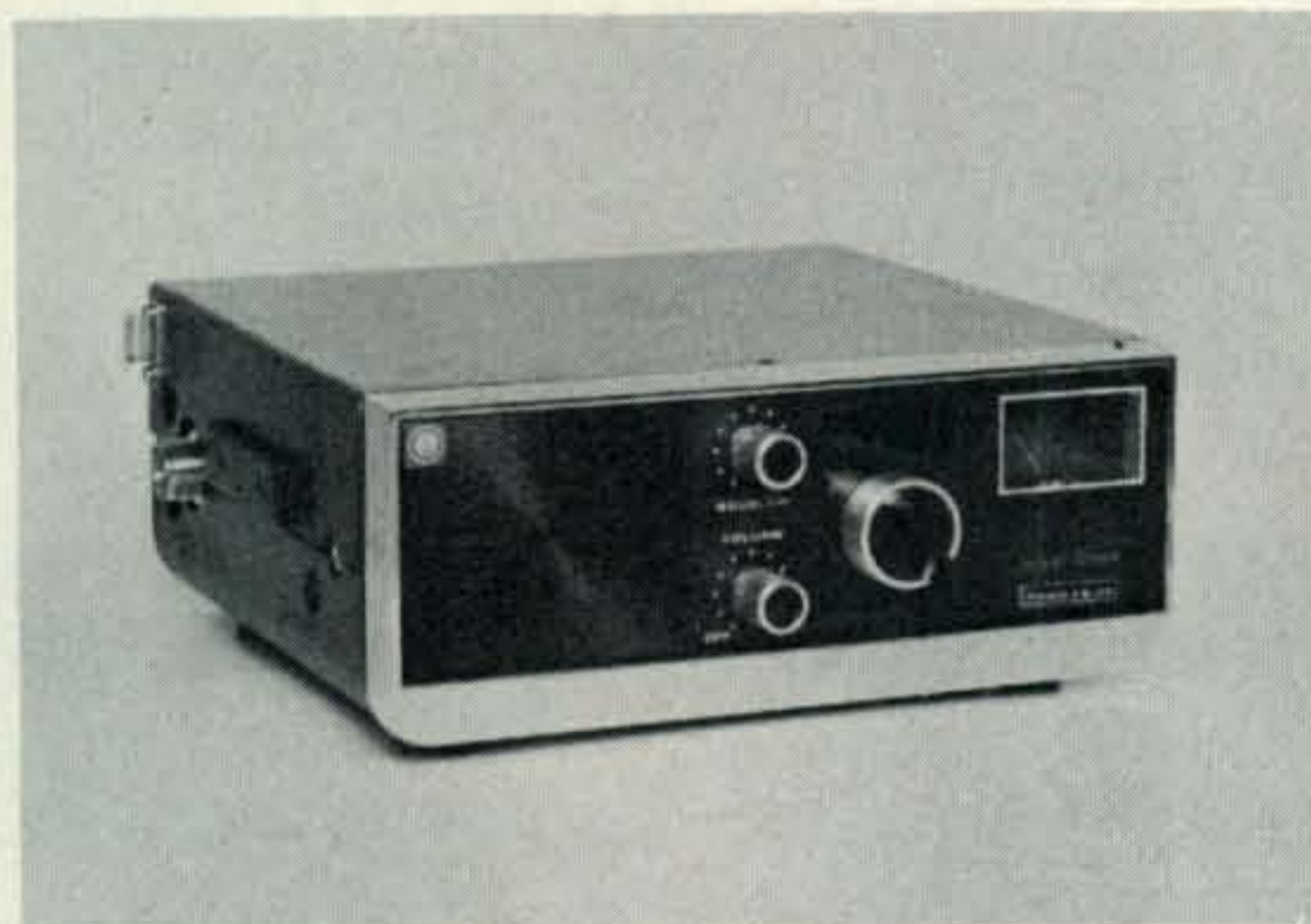
The Swan FM-2X is a 12-channel solid state 2-meter f.m. transceiver designed for amateur use.
