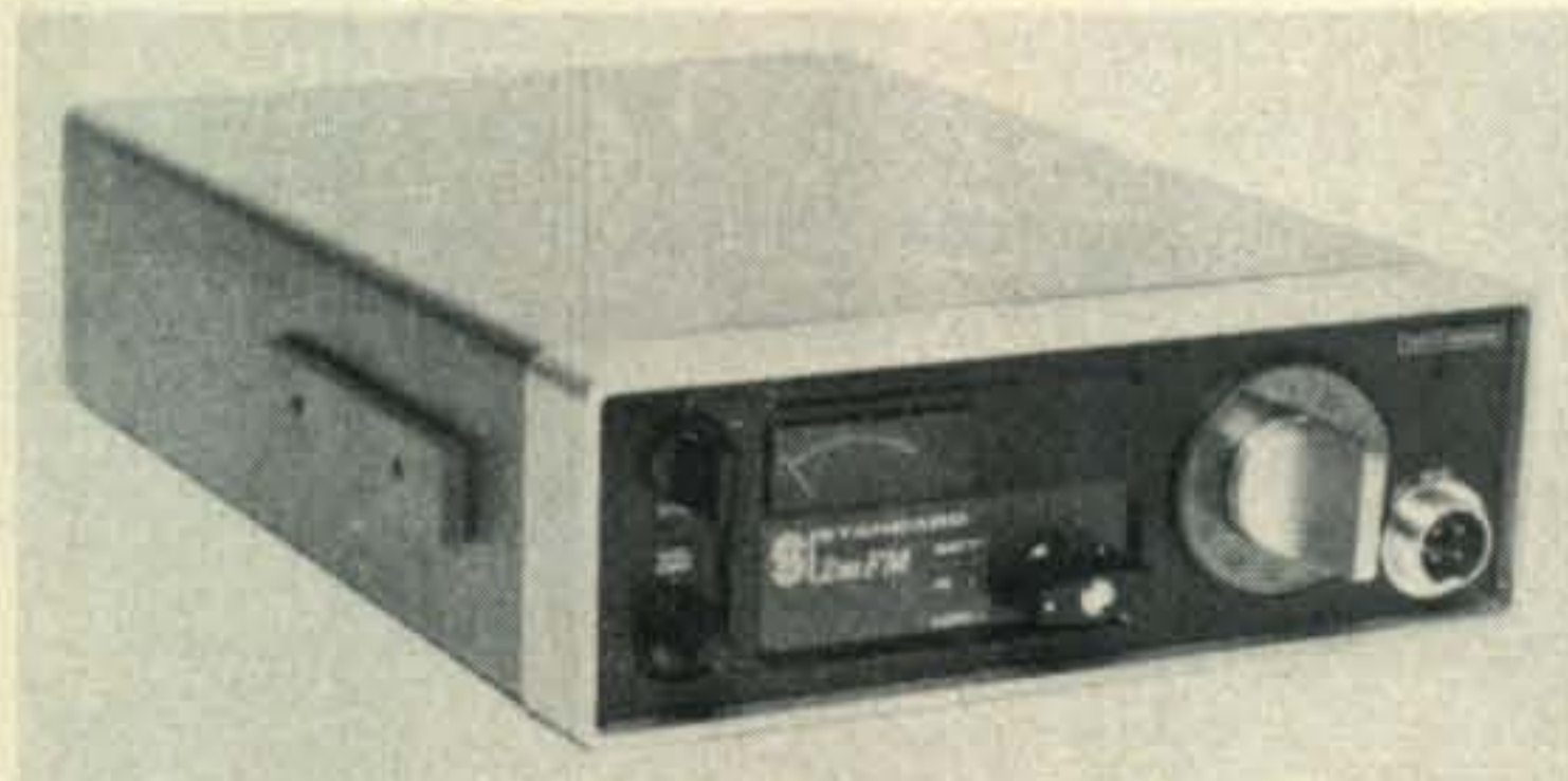
The Standard SR-C826M 2-meter transceiver is a 12 channel, solid state f.m. unit designed strictly for amateur use.
