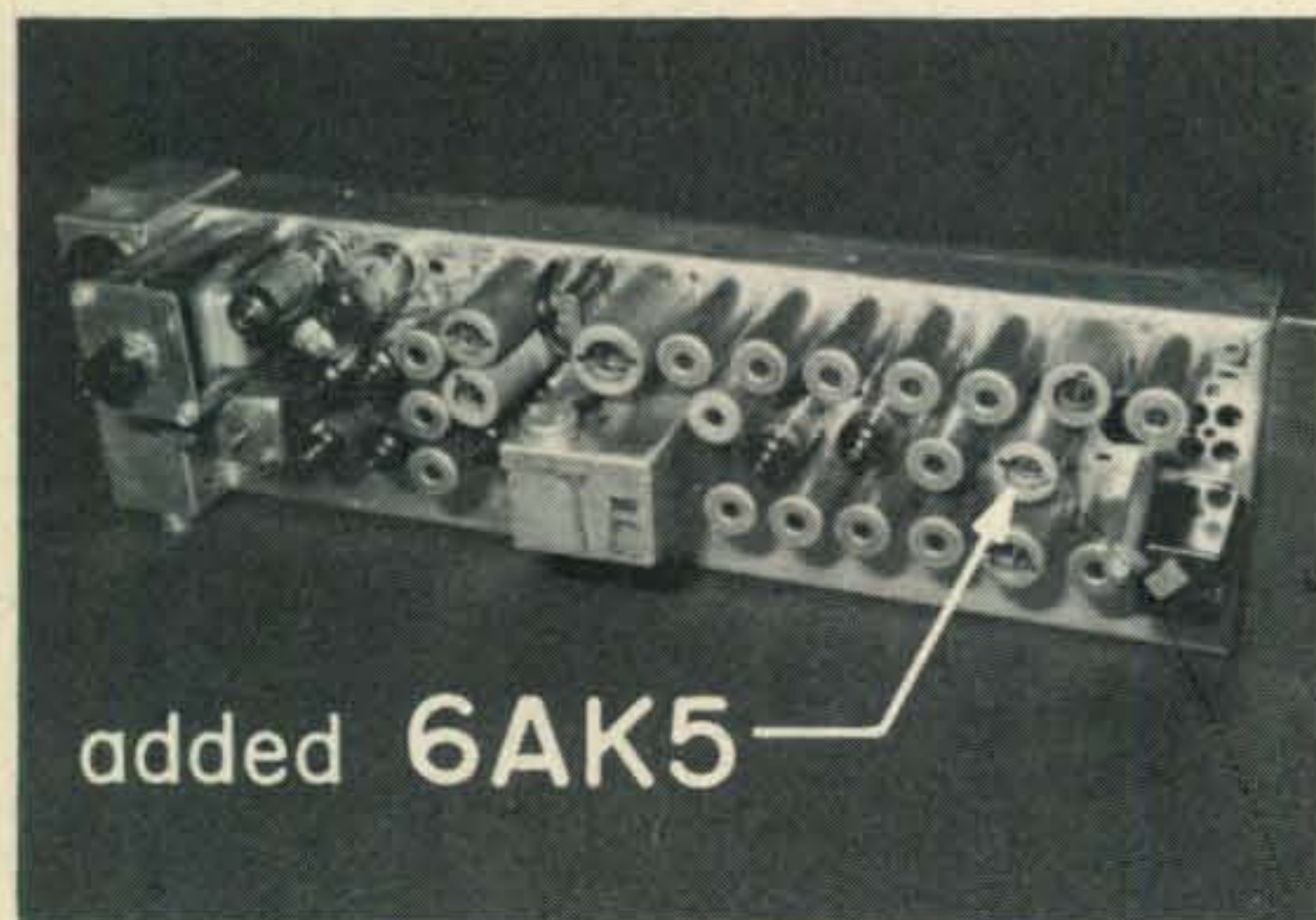
The 225 mc Motorola "G" receiver strip, mounted in an adapter chassis fitted with rack mounting angles.
