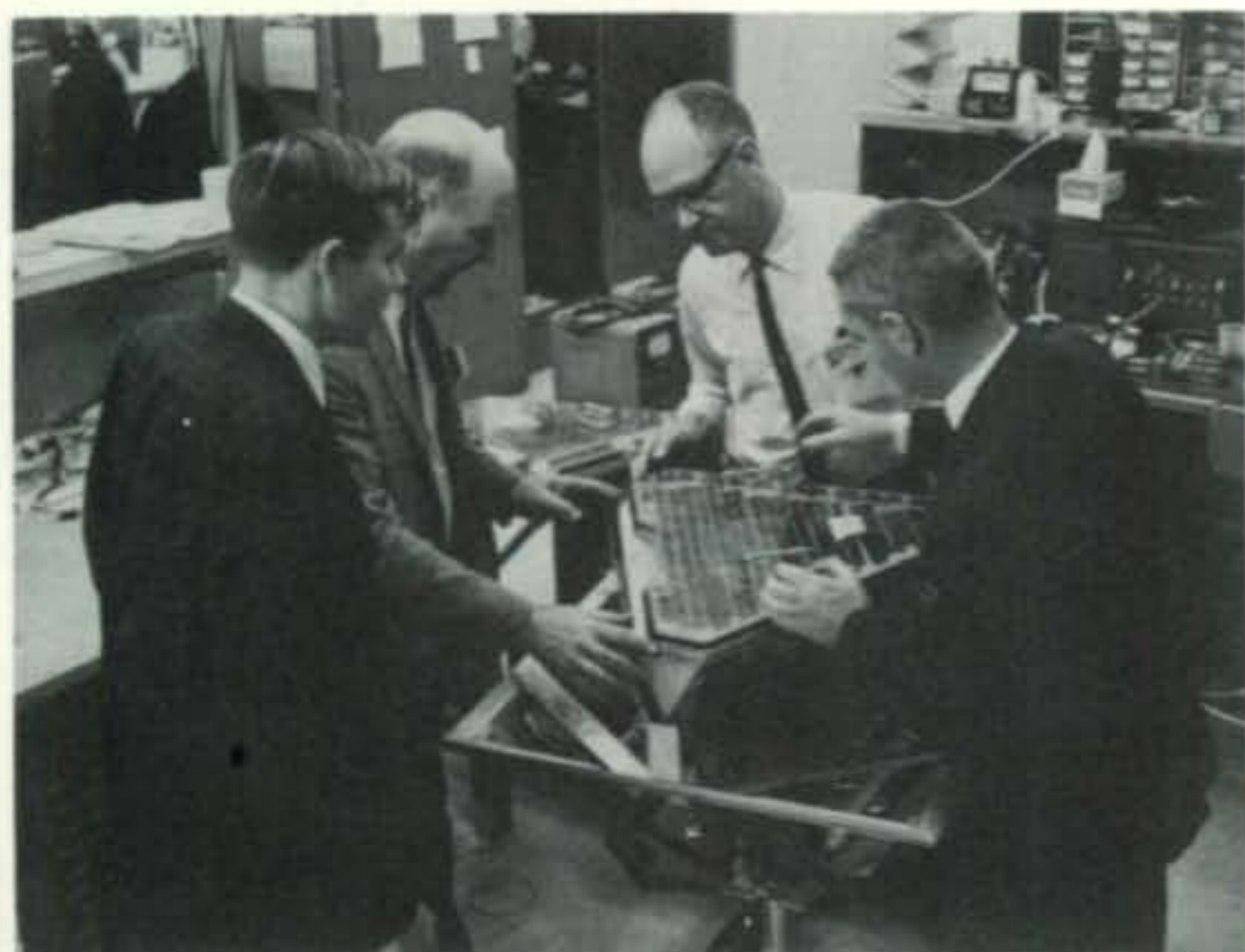
The OSCAR IV satellite undergoes final assembly by some of its amateur builders. OSCAR IV received signals on the 2-meter band and retransmitted them on the 420 mc band after amplification.
