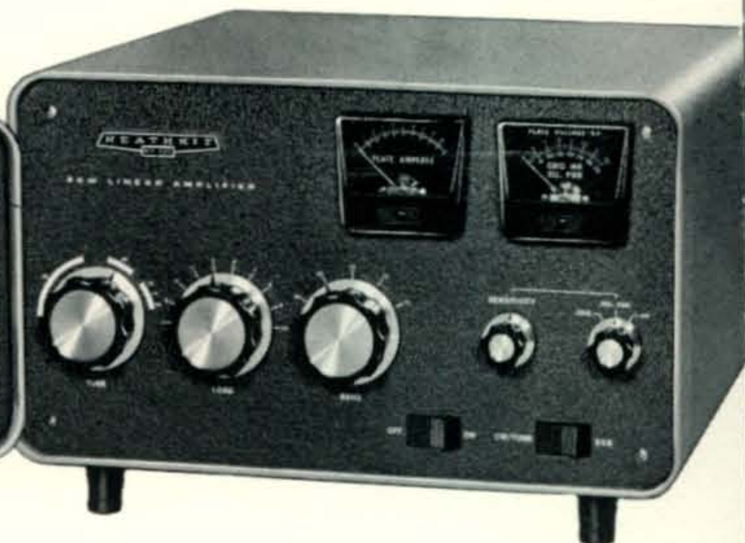
The Heathkit SB-220 Linear Amplifier. 2,000 watts P.E.P. SSB input, 1 kW CW. Just 349.95*
