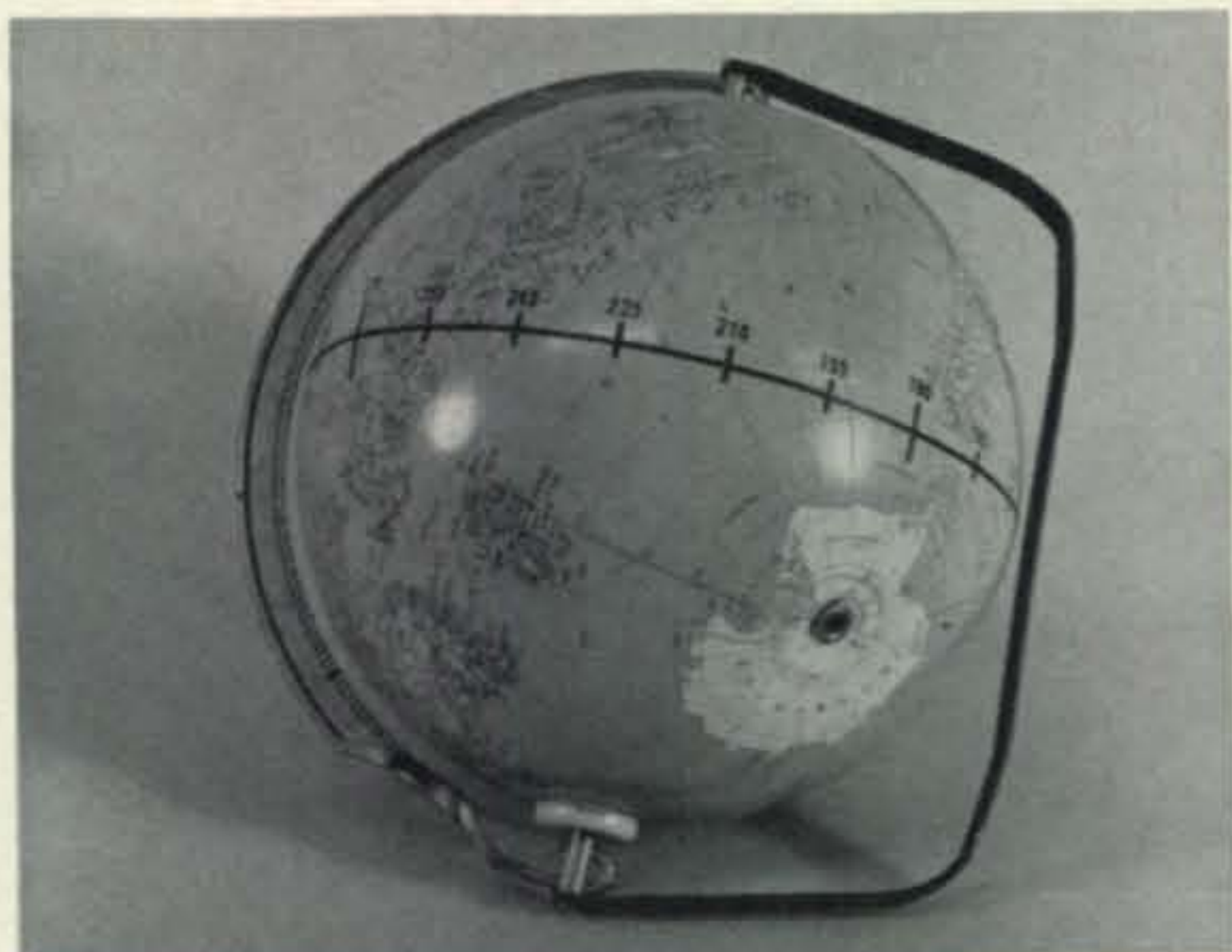
Fig. 4—A new mounting bracket fabricated of flat iron mounts to the original globe bracket.
