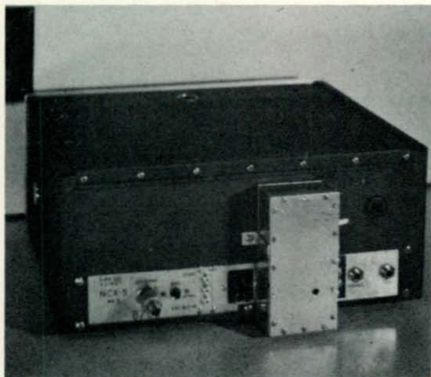
The crystal calibrator shown mounted in position at the rear of the author's NCX-5 transceiver.
