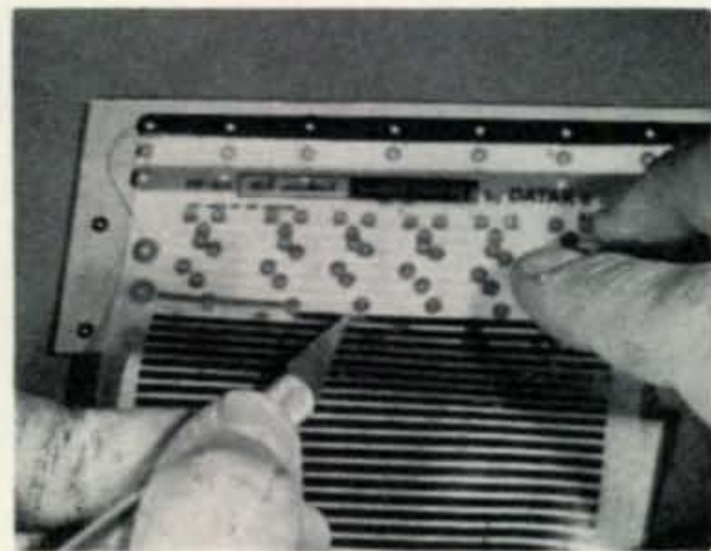
Fig. 3—Cut dry transfer lines over foil, not over pad.
