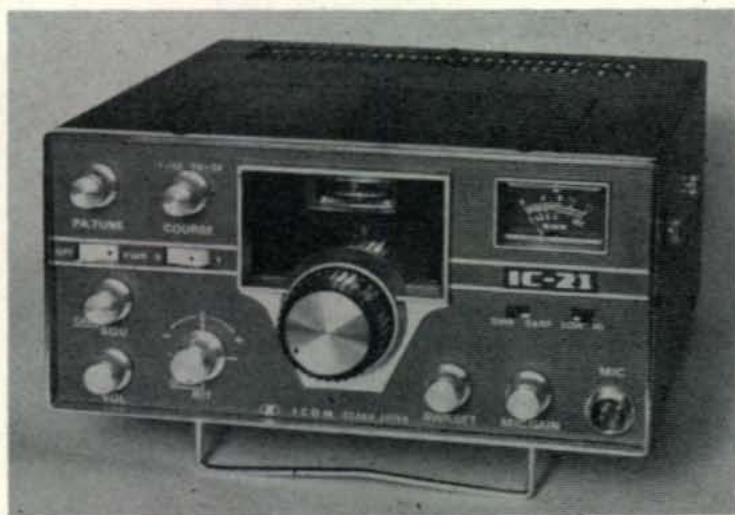
The Inoue IC-21 is a 24 channel, solid state, 2 meter f.m. transceiver. Note how the styling is along low frequency s.s.b. transceiver lines.
