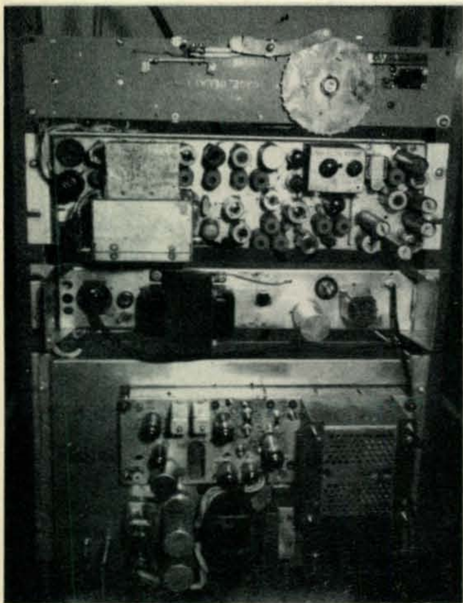
Internal view of the Big Spring, Texas repeater. It consists of a Bendix Mobile unit converted for repeater use. Object in upper right is code wheel lid. (Photo courtesy WA5KHU)
