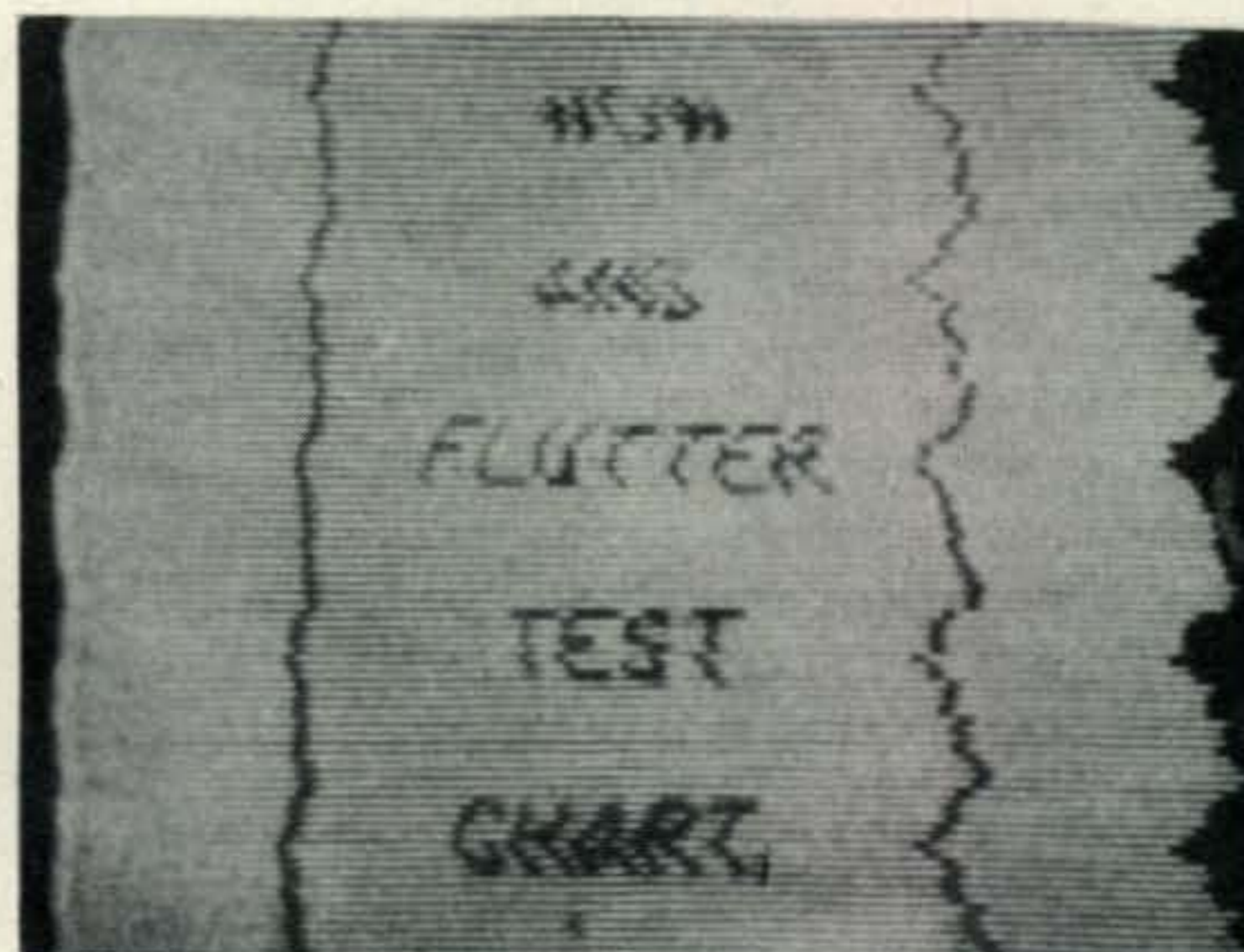
Extreme picture distortion cause by tape recorder with severe “wow.”
