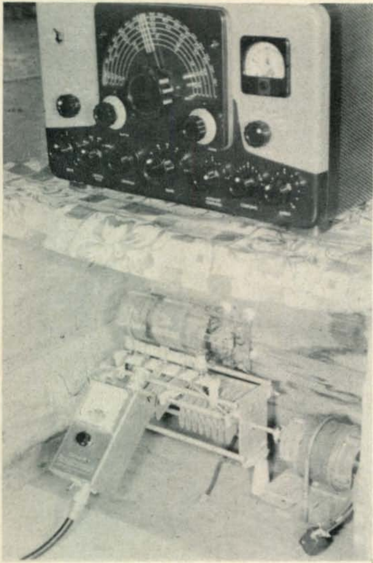
Partially assembled "dog house" for remote antenna tuner. Transmitter is used for initial tune up of antenna. The s.w.r. bridge is then transferred into the shack. Use Viscolene builder's plastic to cover box.
