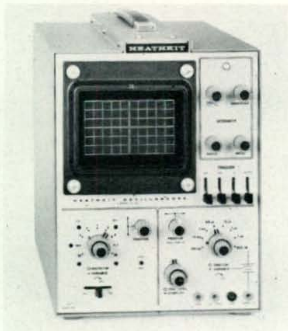
The Heathkit Model IO-103 solid-state triggered-sweep 10 MHz oscilloscope.
