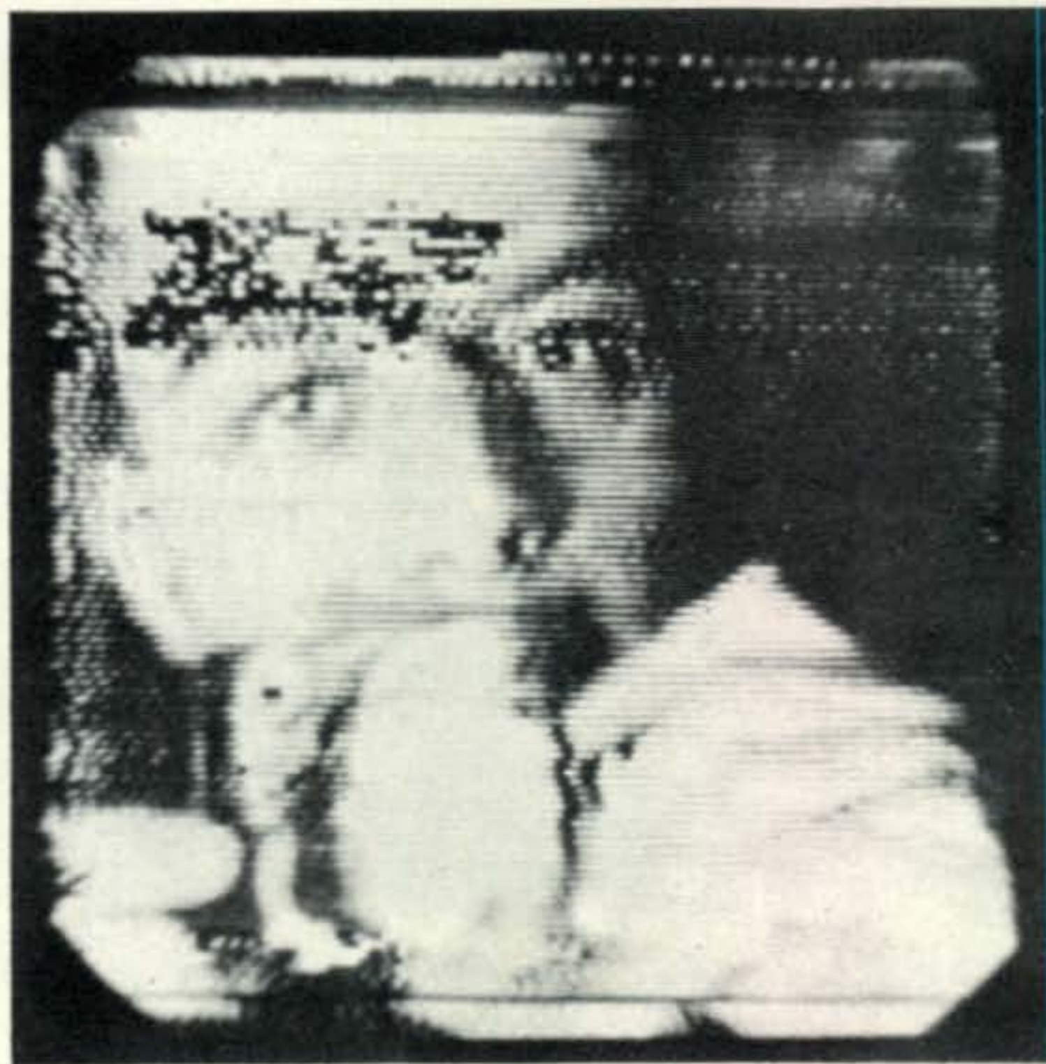
Fig. 3—"Selective fading" type multipath propagation causing cancellation of the transmitted frequency as the forehead was scanned.
