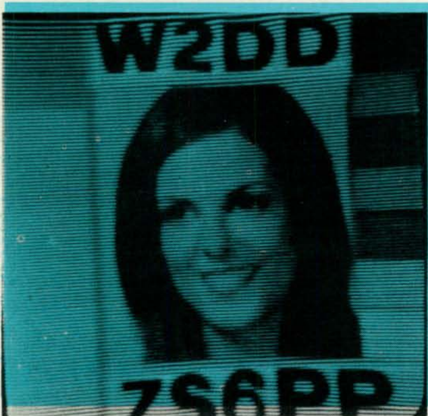
Fig. 2—Single color exposures produced by photographing the red, green and blue. Tape playbacks through corresponding filters. Closed circuit.
