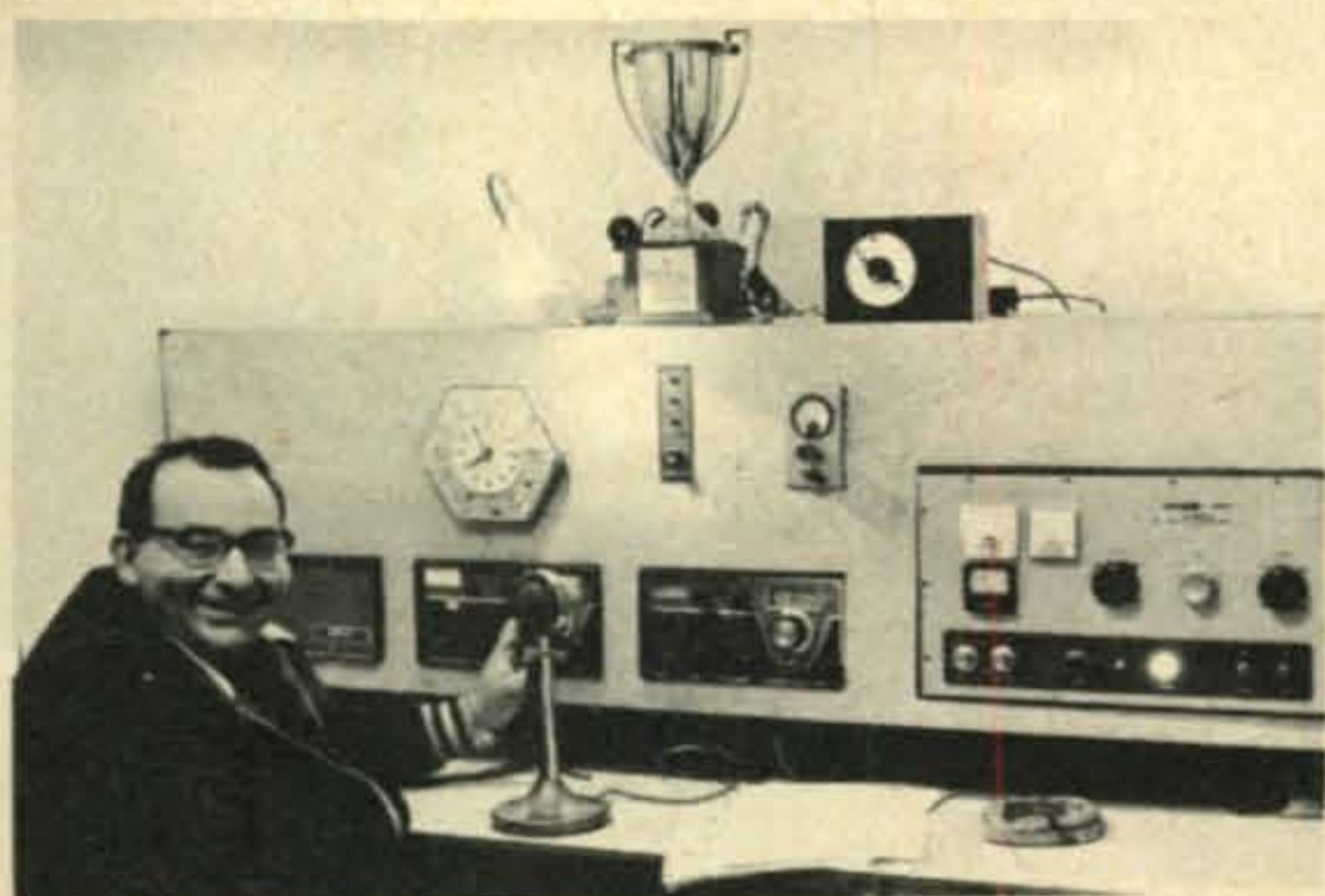
Joe Liberson, Chief Operator at 4Z4HF, the club station at Kibbutz Sasa, Israel. The new shack is located in the highest portion of the kibbutz on top of a 3000 ft. mountain in northern Israel. A 40 ft. home made tower on top of the building supports a three element tri-band beam. (Photo courtesy of K2BYB).
