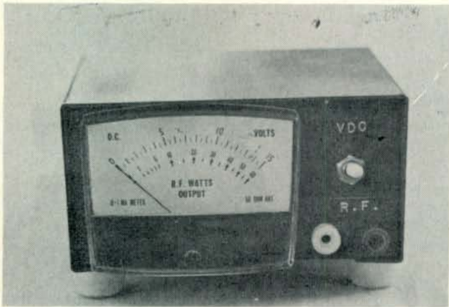
Front and rear views of the simple r.f. power meter for mobile use with the author's 2-meter f.m. transceiver. The phono jack on the rear panel connects to the r.f. sensing unit at the trunk-mounted amplifier. Note the shaft lock used on the calibration control to prevent accidentally changing its setting. The cabinet is an LMB 342, 3 \times 4\frac{1}{4} \times 2\frac{3}{8} ".
