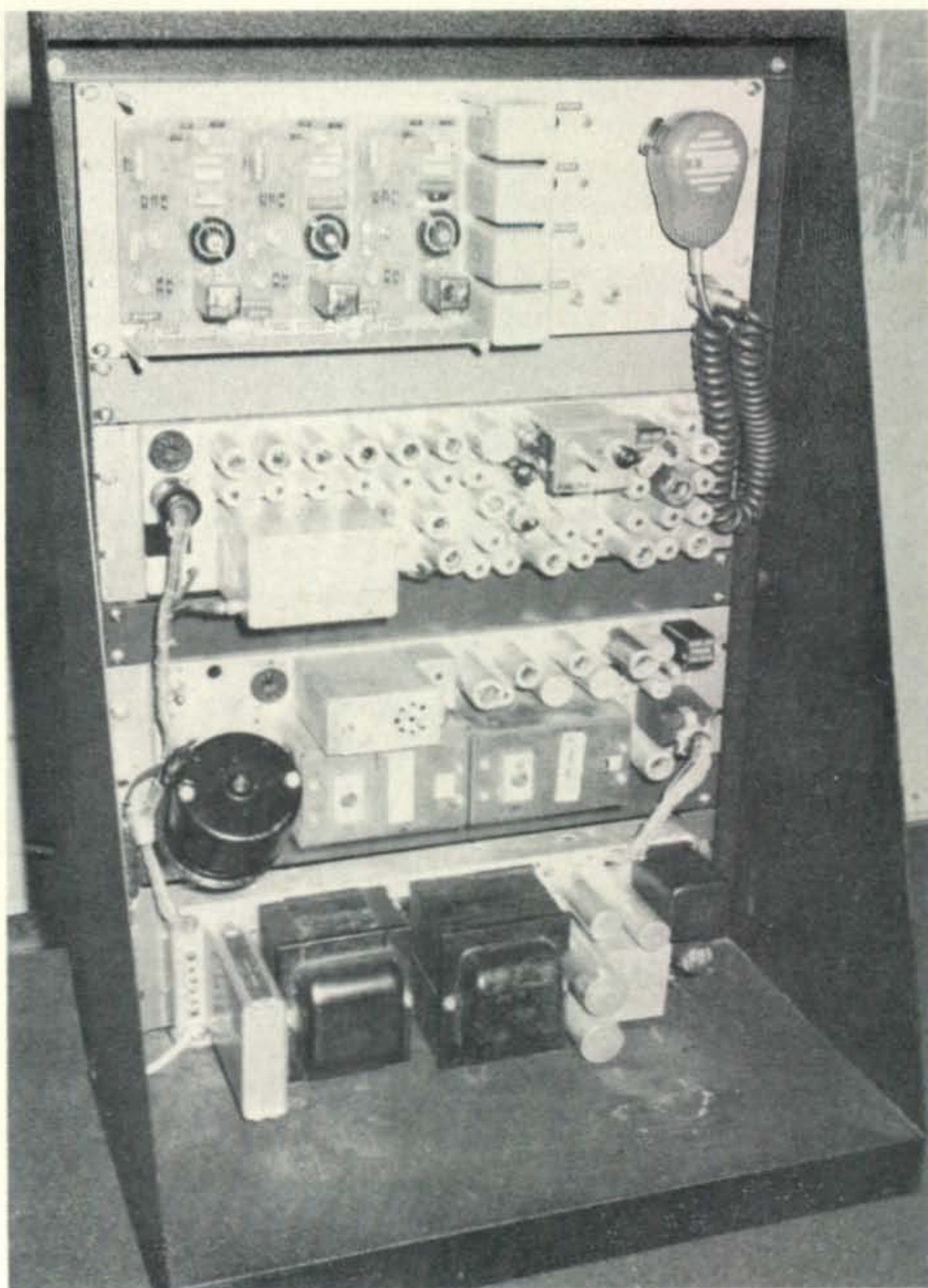
Fig. 12—Control station for the RTTY repeater, mounted in an open table-top rack. The Control Unit is at the top (with dust cover removed). Next is the 52.60 MHz low-band monitor receiver; next is the T44 u.h.f. transmitter. The a.c. power supply for the receiver and the transmitter is at the bottom.
