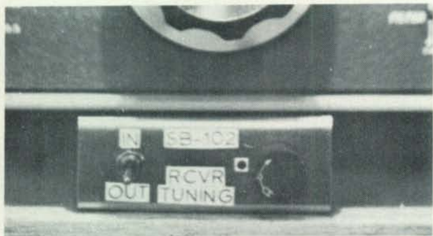
The receiver-only tuning adapter is held beneath the SB-102 and requires no permanent changes in the transceiver.
