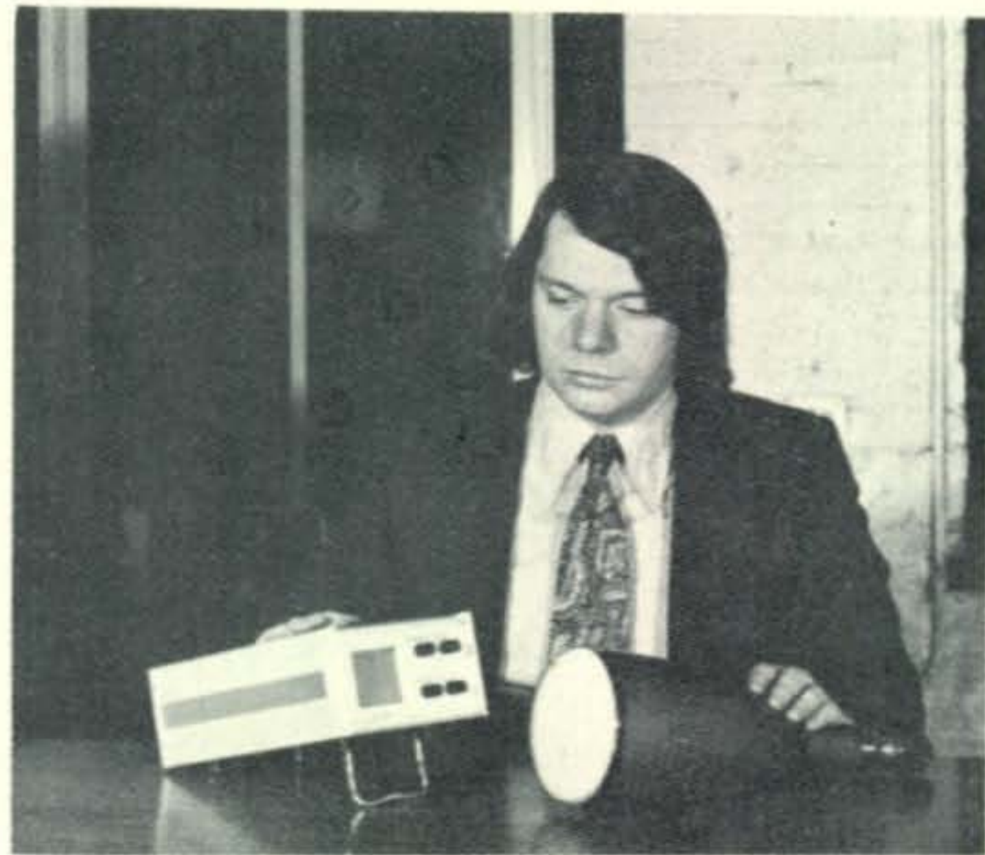
The author compares the compact SS Mark 4 slow scan TV monitor with a standard 5" electrostatic deflection CRT.
