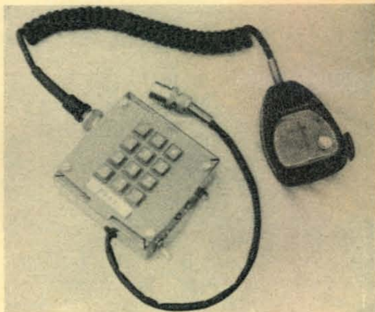
Overall view of the Touch-Tone pad assembly.
