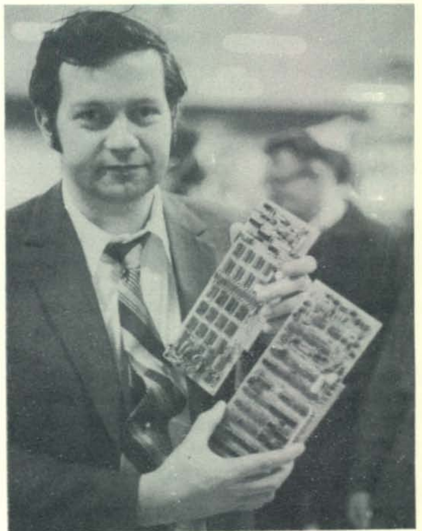
Mike Tallant, W6MXV, holding the signal processing boards for his digital fast-scan to slow-scan converter. His project won first prize in the SSTV homebrew contest at Dayton.
