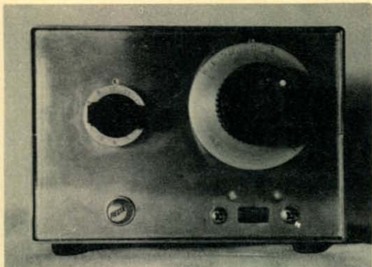
Fig. 2—The h.f. converter has three front panel controls: Bandswitch (left, marked in MHz); R.F. Tuning (large knob with H and L skirt markings corresponding to Hi and Lo ranges); and Hi and Lo Range switch (slide switch selects r.f. coils for Hi—5-18 MHz or Lo—2.5-6.0 MHz ranges). Emblems on this and other units are fabricated from stainless steel and finished in black and red.
