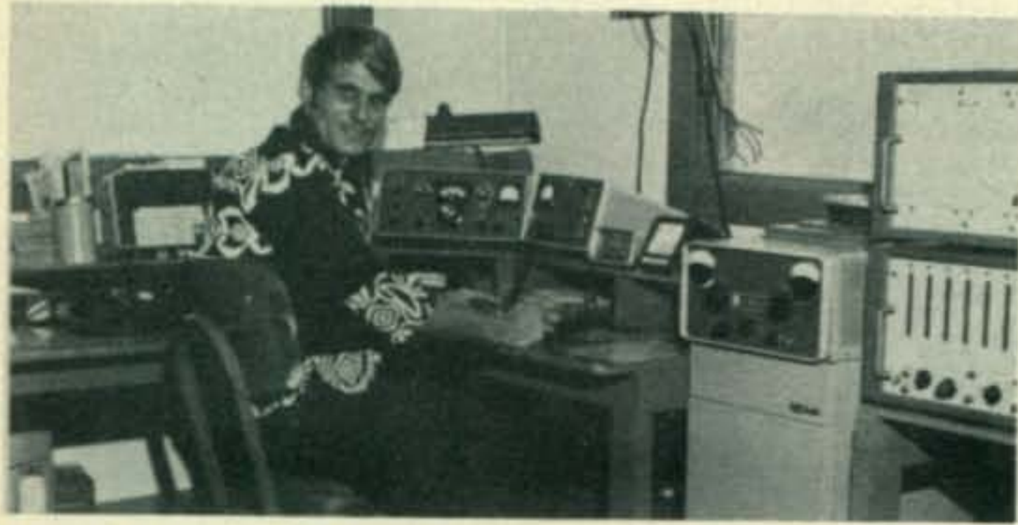
Tom French, KG6JBG, operating the big rig at club station, KG6ALV, near the south coast of Guam. The station has a complete S-line, a Henry 2KD-2 linear, a 3-wire Rhombic towards California and a TH6DXX beam.
