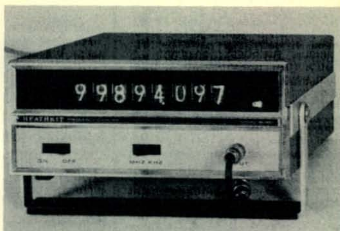
The Heath IB-1102 Frequency counter shown with a readout of 99,894.097 kHz (99.894097 mHz) for a resolution to 1 Hz with the kHz range in use as indicated by the lamp at the lower right of the viewing window.
