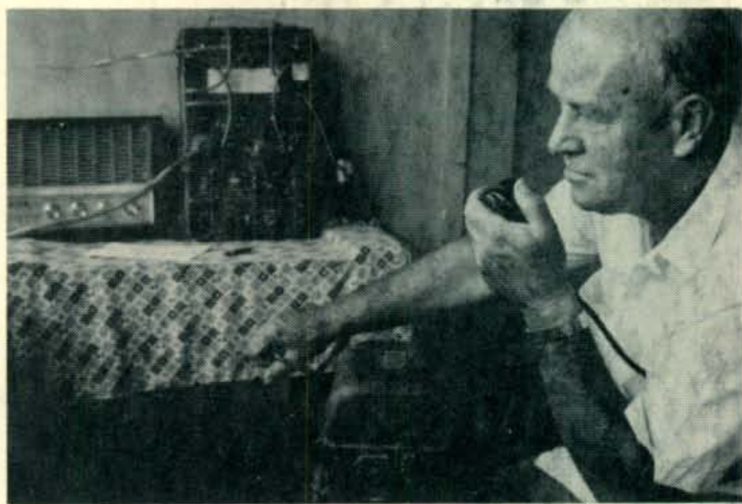
Missionary uses surplus WW II crank generator to power an ancient BC-1306 transmitter/receiver to maintain daily skeds with other missionaries.
