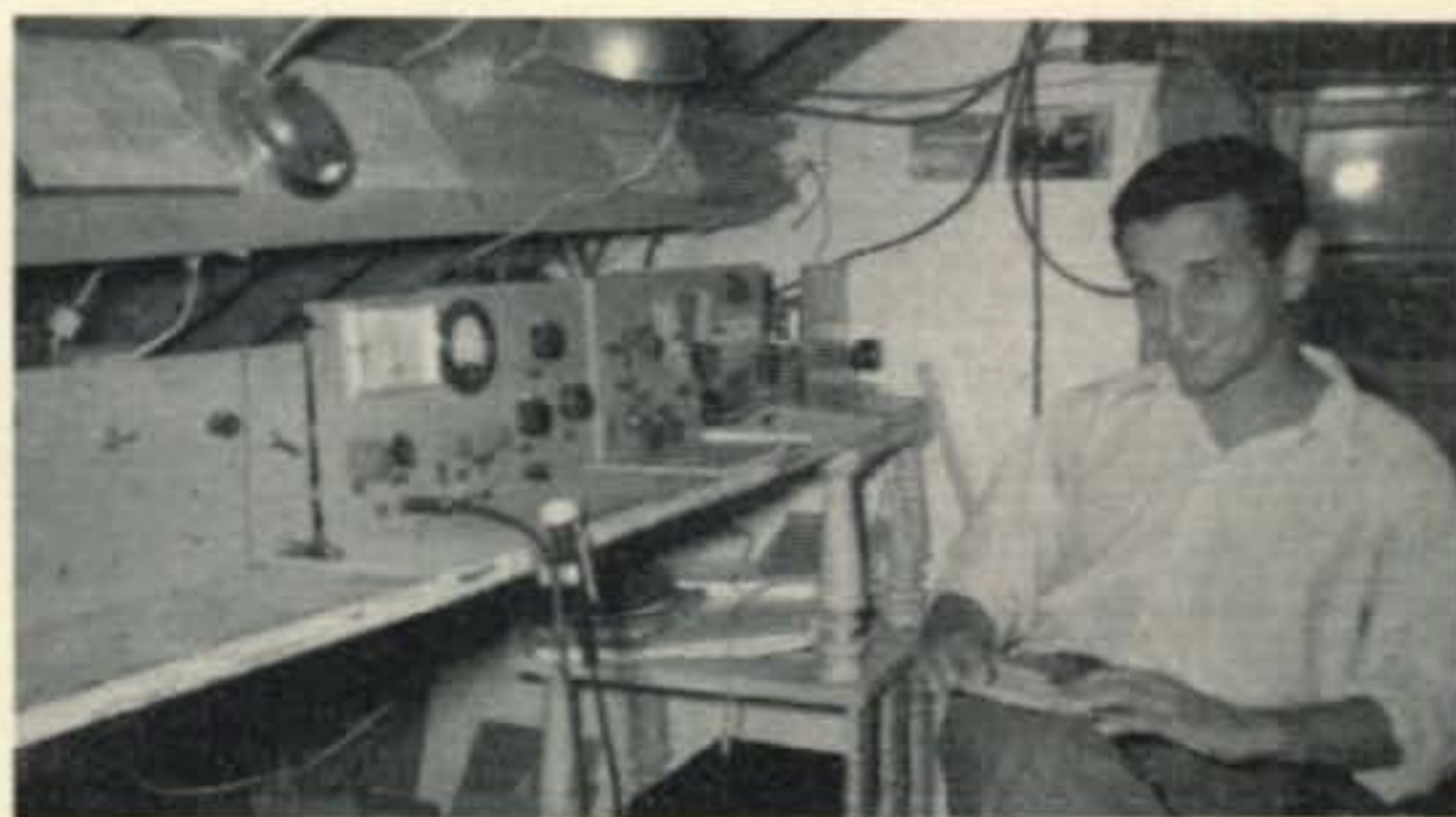
Jorge H.A. Da Costa, CT2BA, of San Carlos, Terceira, Azores. Jorge's rig includes a homebrew transmitter with a BC-348 receiver. (Photo via Jake, CT2AZ)
