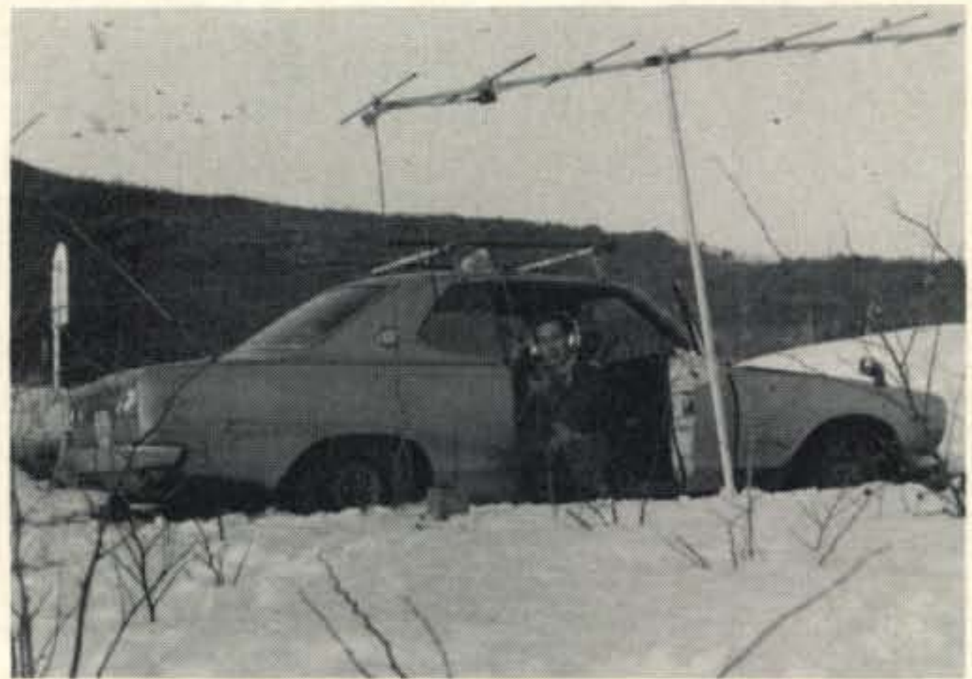
JA1VDV/JAØ shown operating through OSCAR-6 from his mobile station in snow covered mountains north of Tokyo. Several stations were worked using 10 watts and the 7-element horizontal Yagi. A 10-meter wire dipole was used for receiving.
