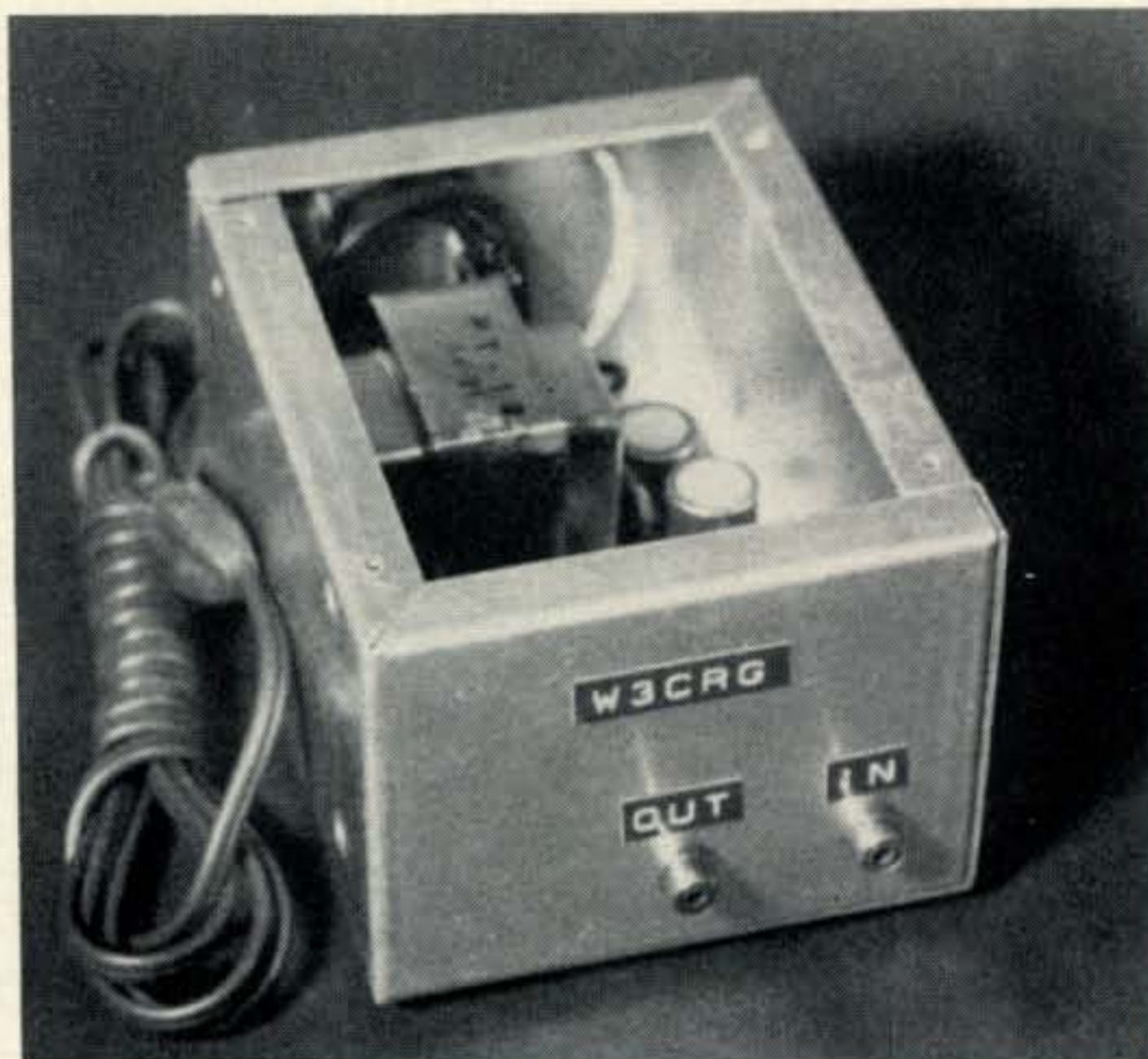
The scaler is completely self contained in a 3" × 4" × 5" aluminum cabinet, with its own power supply.
