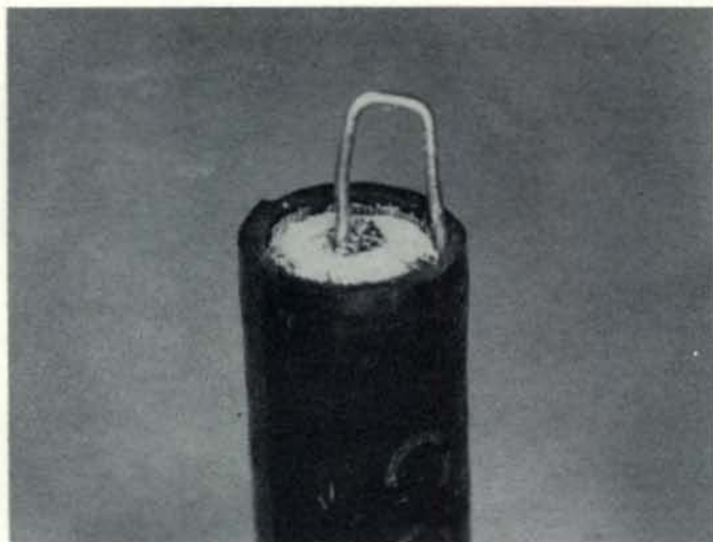
Fig. 3—Hairpin type of short on open end of coax. Make it as short as possible while still giving a perceptible dip.
