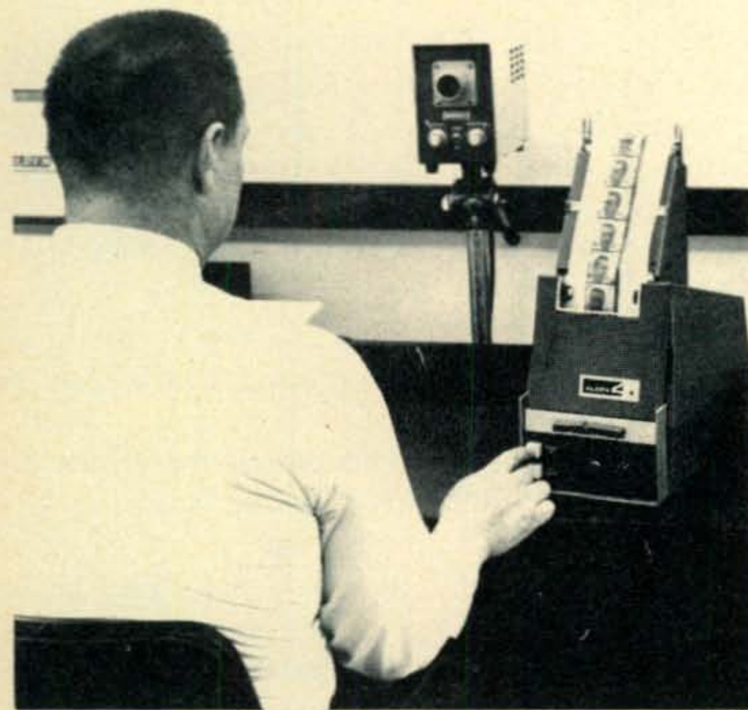
The Alden 400 hard-copy SSTV recorder as it reproduces the output of a Robot camera.
