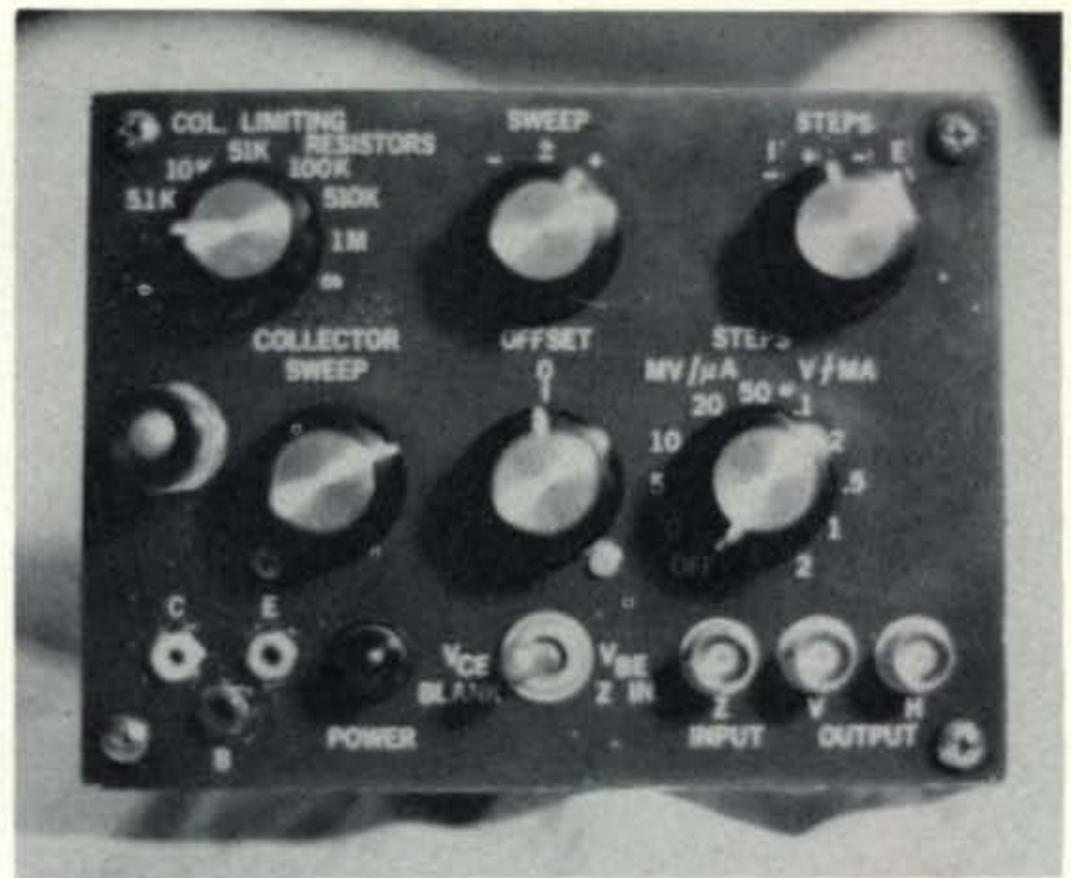
Front panel of the curve tracer showing control locations and designations. The knob at left center is a lock for the plug-in module. The "Z-Input" BNC connector near the lower right is not used for curve tracer functions.
