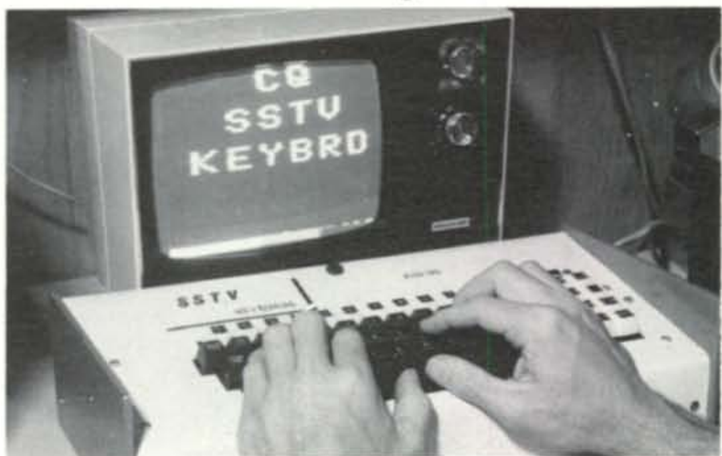
18 characters (including blanks) have been entered into the SSTV keyboard memory so far.
