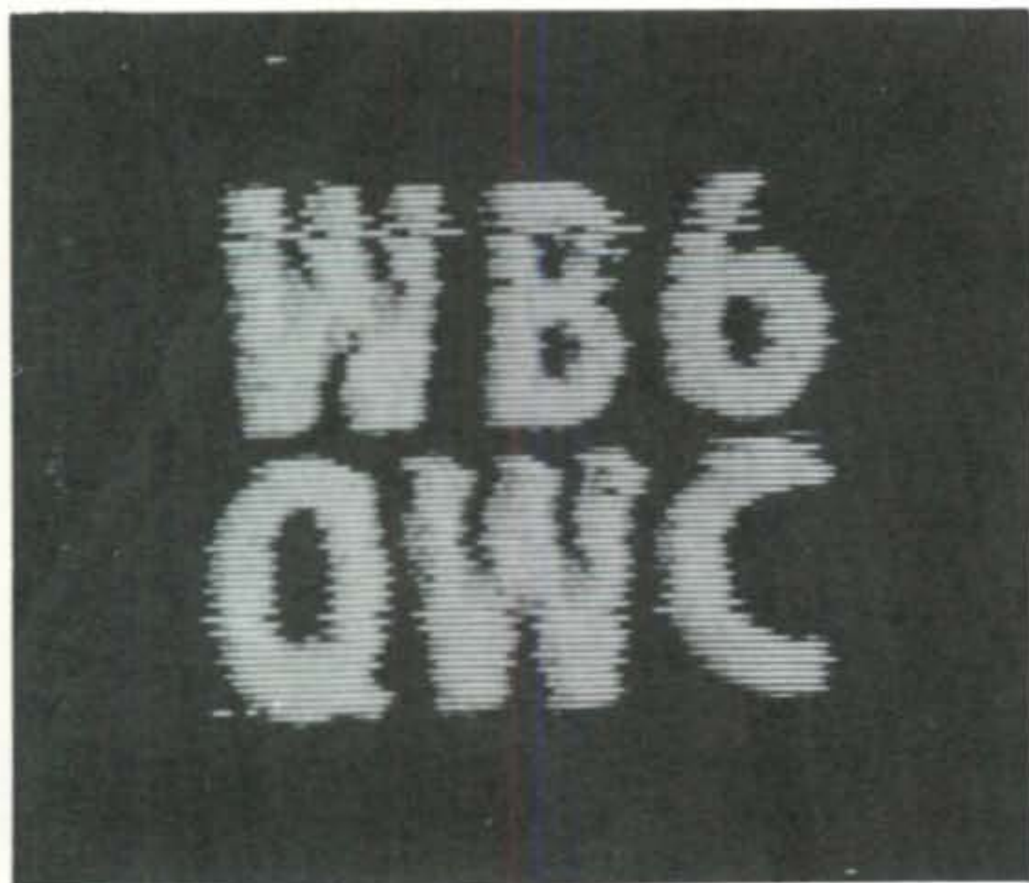
Fig. 1—Example of line-to-line jitter or staggering.
