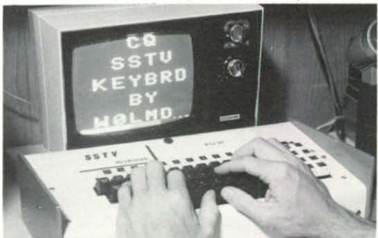
All 30 characters have now been entered into memory. The characters will be continuously outputted until either the erase key is pressed or power is shut off.
