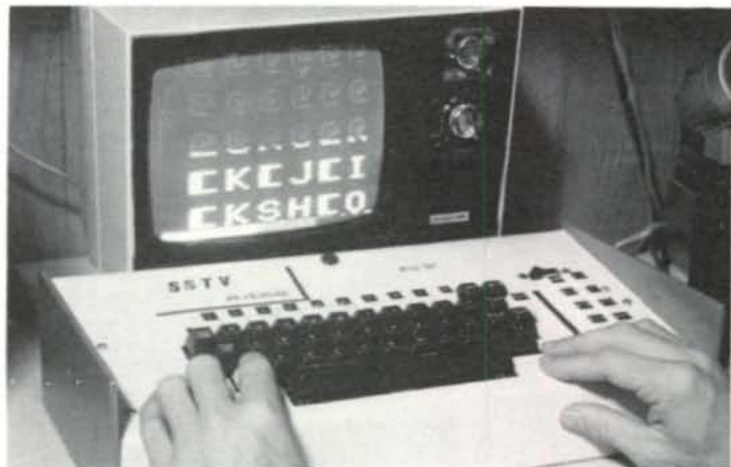
Keyboard has just been powered up. Erase key has been depressed, and the SSTV screen is clearing.
