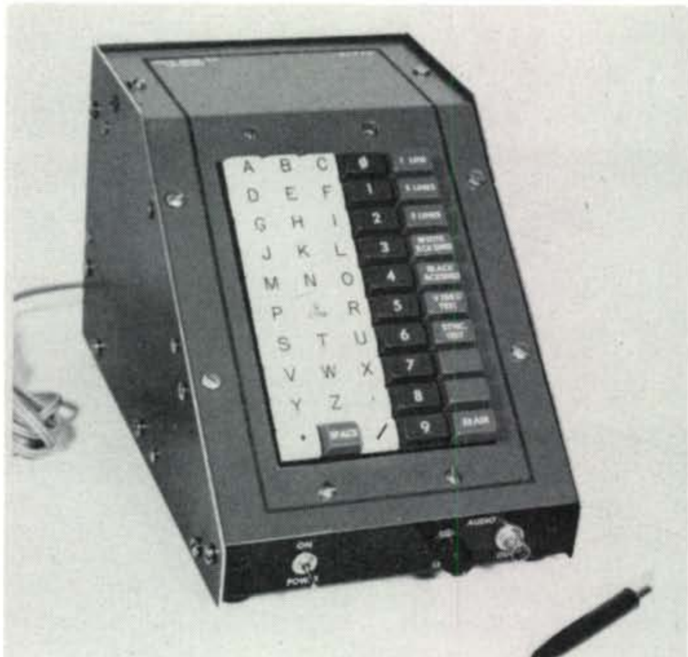
SSTV keyboard built by K7YZZ using an old stock market keyboard.
