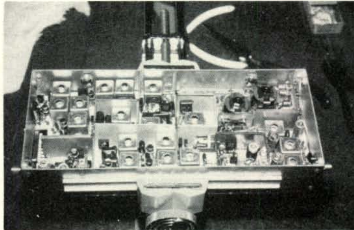
A close-up view of OSCAR 7's 2-to-10 meter repeater module undergoing final testing before assembly. It was built by AMSAT under the direction of Dick Daniels, WA4DGU.
