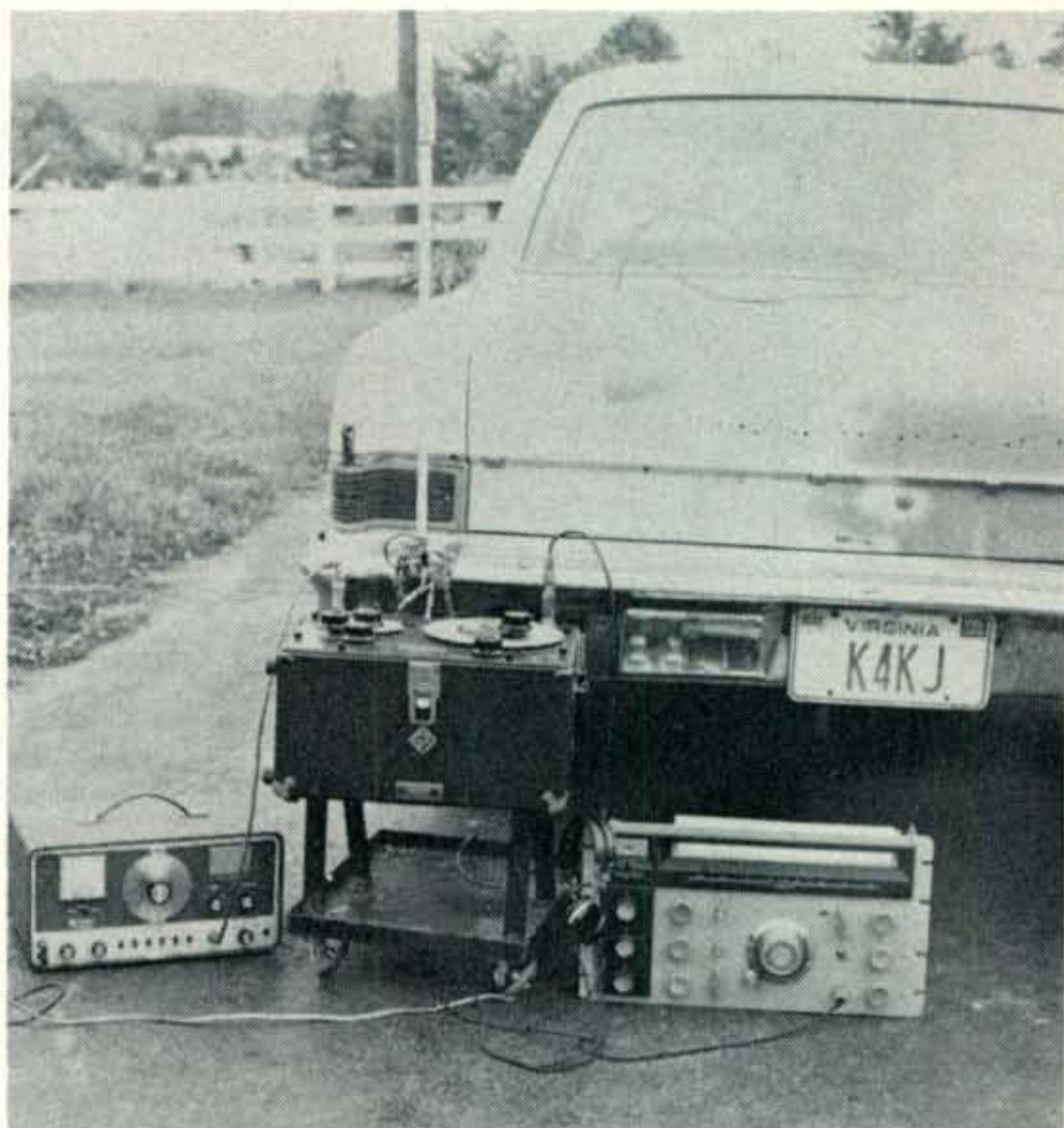
Fig. 12—Test set-up for measuring the antenna impedance of a mobile whip.
