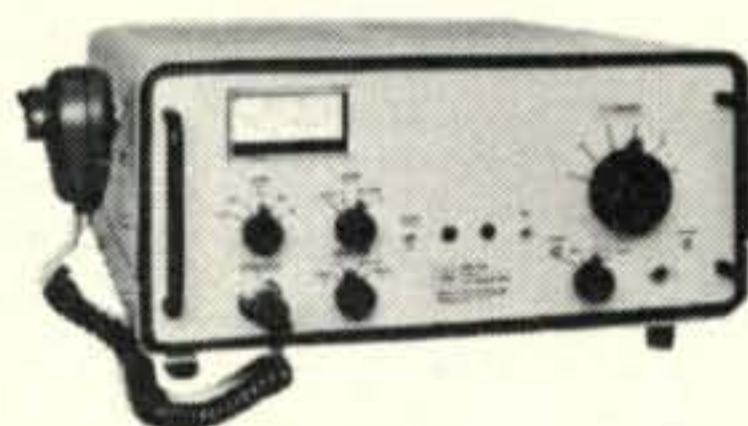
AN/URC-77 150 W SSB TRANSCEIVER
