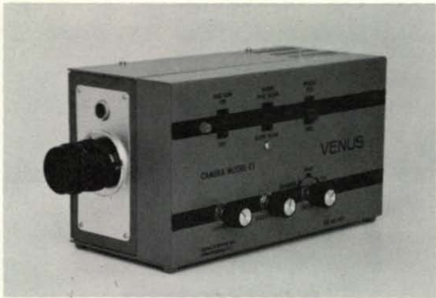
Fig. 2—The Venus C1 Camera in position for slow-scan TV pickup.
