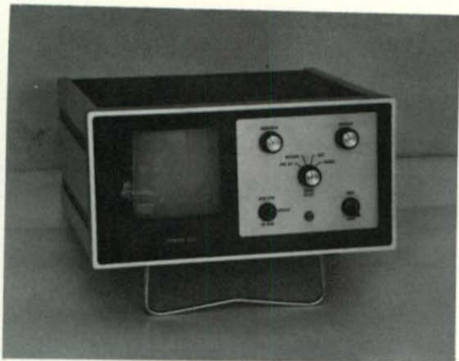
The Venus SS2 Slow-Scan TV Monitor. The bail under the monitor will fold if desired to allow the monitor to sit flat.
