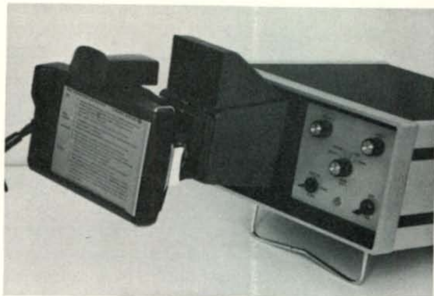
Polaroid "Colorpac" camera and Venus P1 Polaroid Camera Adapter as used with the SS2 Monitor.
