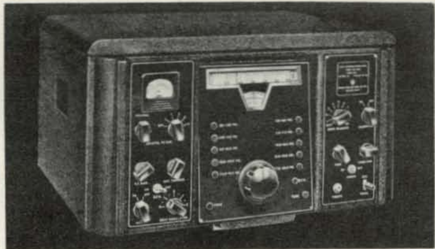
Fig. 5—The Millen DPF-501—the deluxe receiver that never left the drawing board. Weighing 107 pounds and having direct dial calibration and general coverage to 41.5 MHz, this receiver was the result of years of design work by Jim Millen. Unfortunately the advent of s.s.b. and soaring production costs doomed the DPF-501 and it never was built in quantity.
