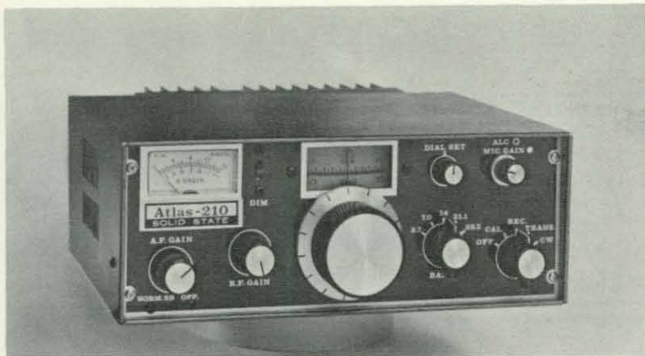
Front view of the Atlas 210 solid state transceiver. Despite the small size of the unit, all controls are full size and easily manipulated.
