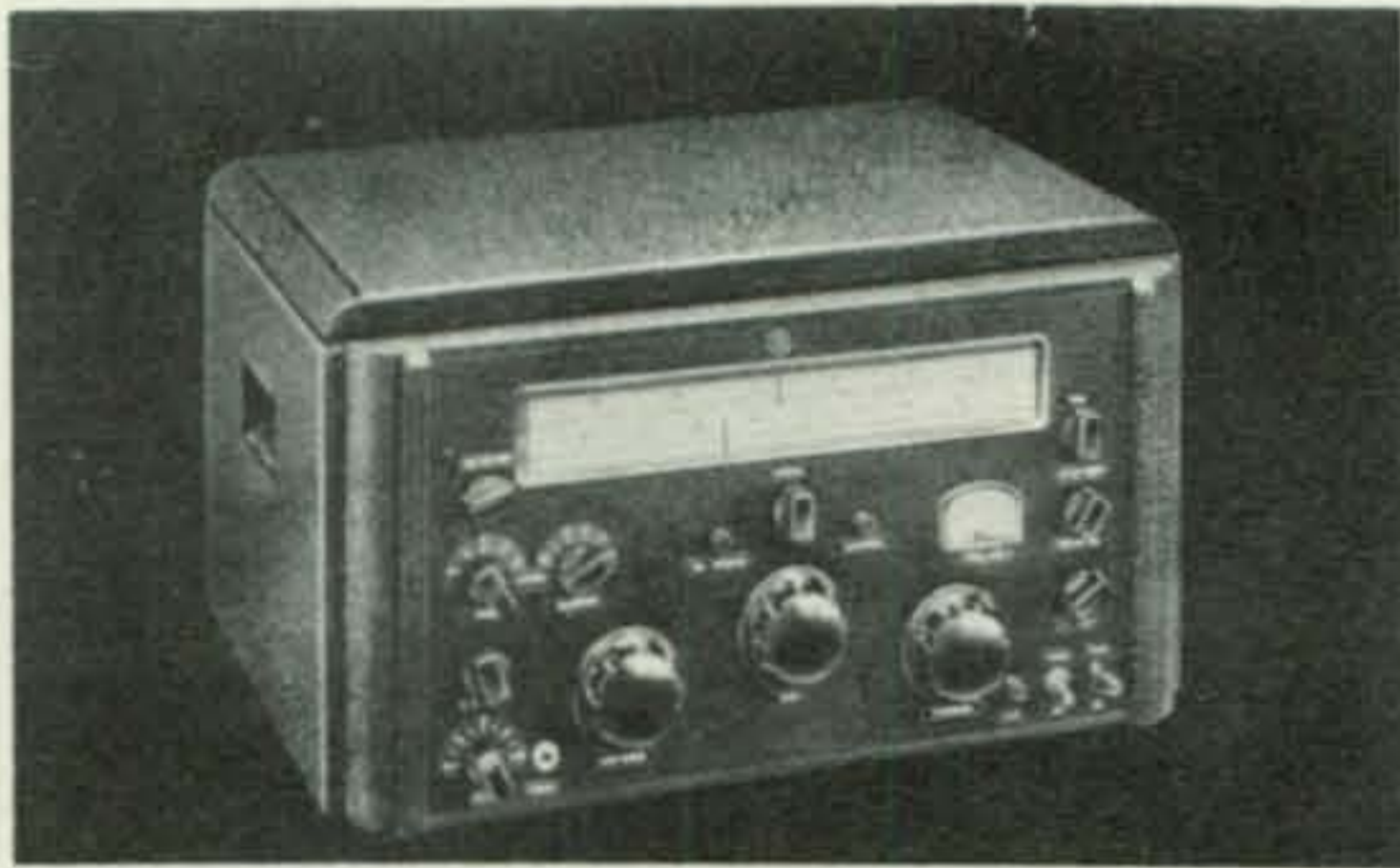
Fig. 4—The Millen DPF-201—the receiver that never was! This was a double conversion receiver covering 550 kHz to 31.5 MHz. A directly calibrated slide rule dial was used, with auxiliary bandsread tuning for all amateur bands. A 6AK5 r.f. stage was used, and the receiver included an antenna compensator for exact alignment of the r.f. stage. The DPF-201 employed a sliding coil catacomb mounted beneath the chassis and weighed 80 pounds.
