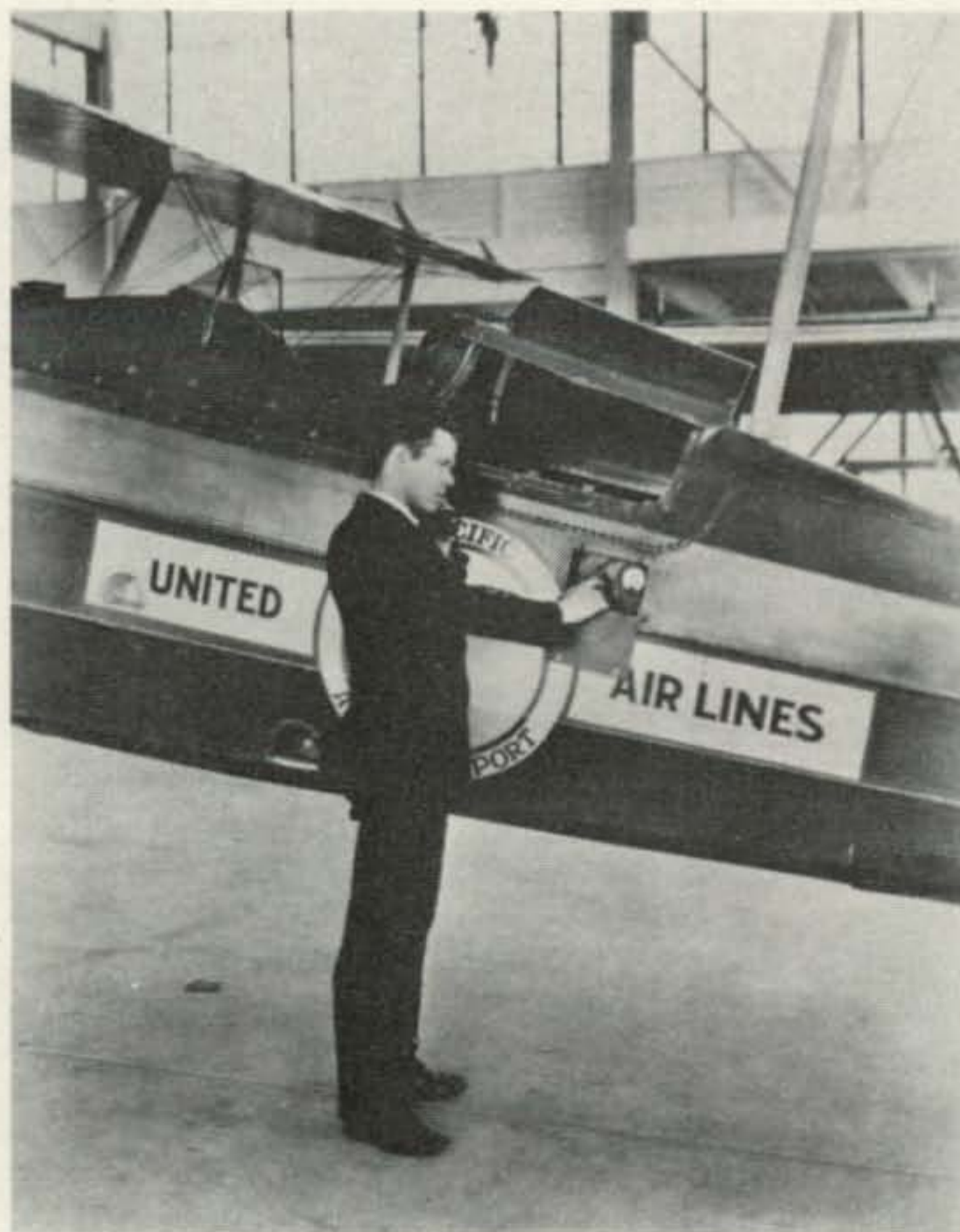
Fig. 1—Flying was a chancy thing in the early "thirties" and aircraft radio was unreliable and heavy. Most airways relied upon beacon lights, placed atop high hills, for navigation. Only two frequencies (3105 kHz and 6120 kHz) were used for aircraft communication in the United States. Here, a ground engineer for United Airlines adjusts a radio transmitter in a mail plane prior to takeoff. The mail compartment is directly above engineer's head.
