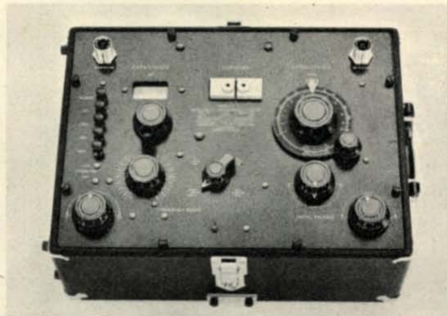
Fig. 1—The General Radio 821-A twin-T impedance measuring bridge. This is a later production unit and uses the GR-874 series connectors for the generator and detector. (Photo courtesy General Radio Co.)
