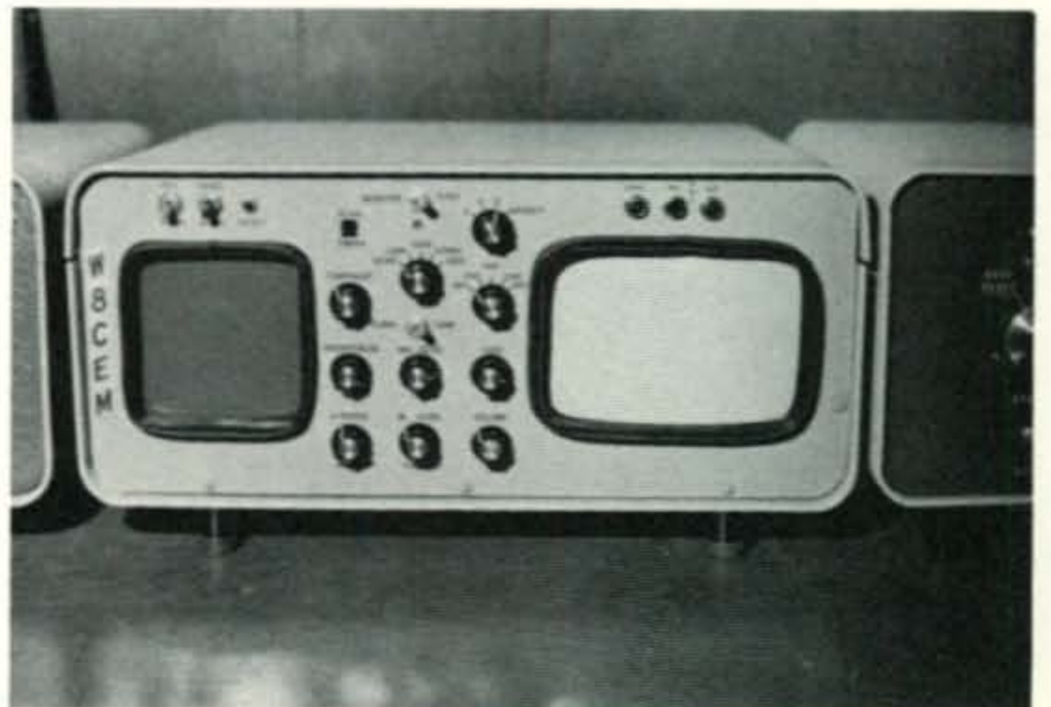
Combination fast and slow scan monitor designed and built by W8CEM.
