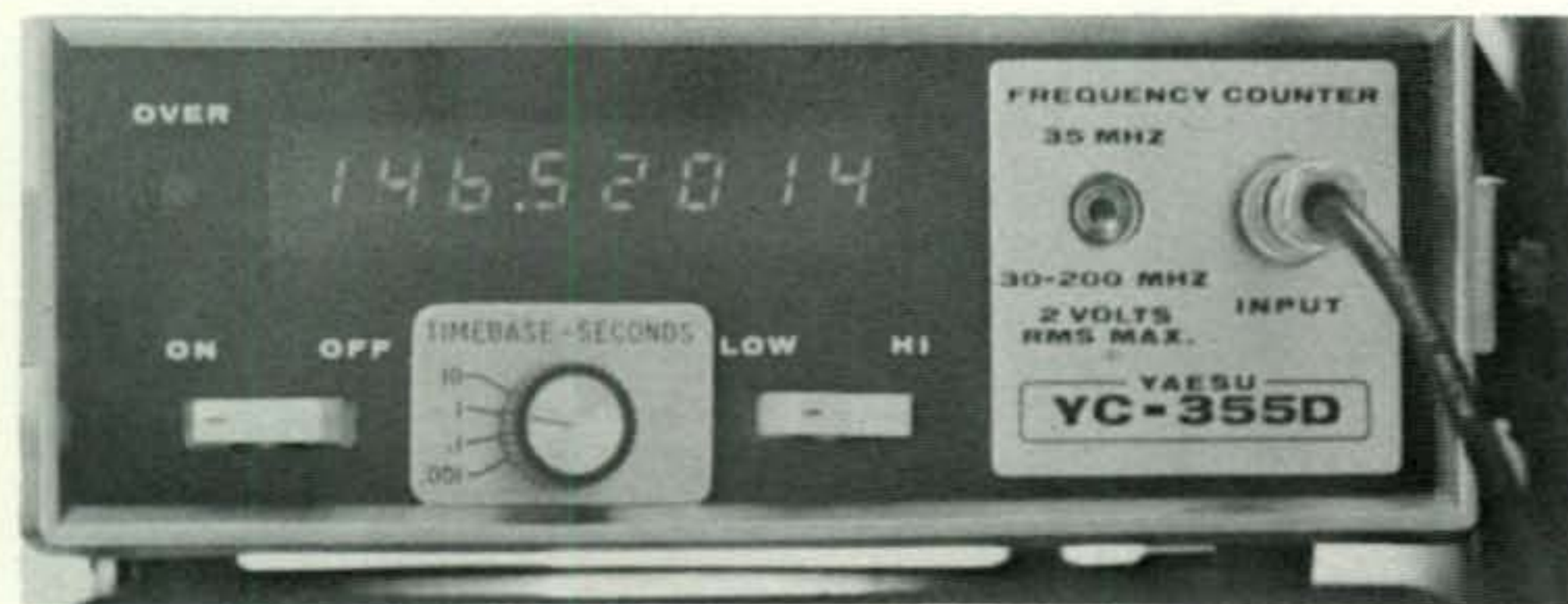
Front view of modified counter. The new switch labeled "Timebase-Seconds" could be more accurately called "Gate Time-Seconds." Switch is in the 1 second position allowing 146.52014 MHz to be read with resolution to 10 Hz.
