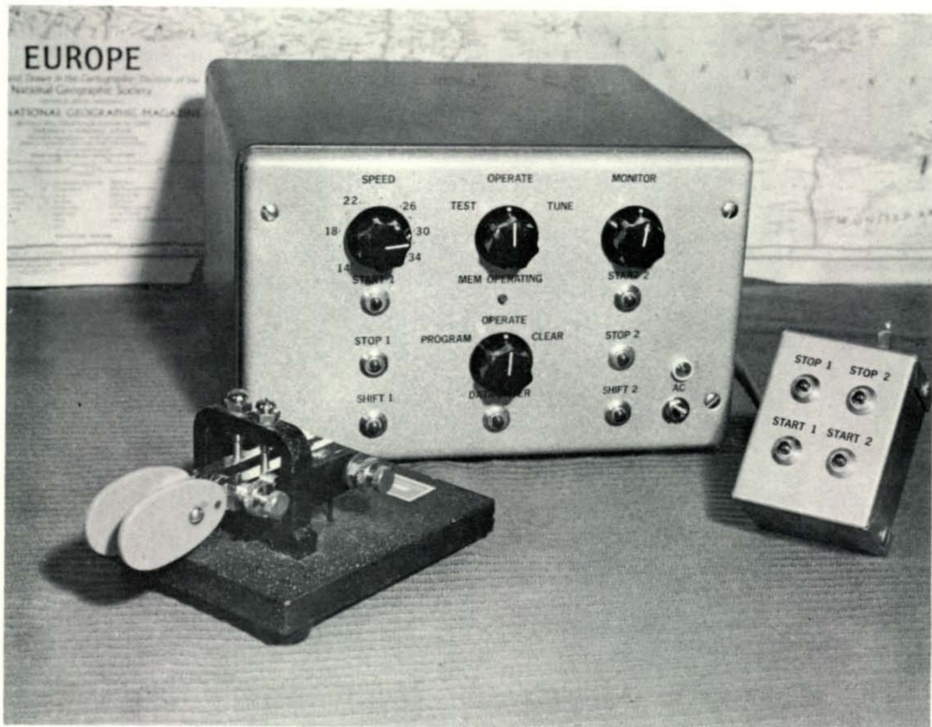
The author's keyer showing the remote switch box and Brown Brothers paddle. Sharp eyed readers will notice two extra push buttons on the main unit and one extra on the remote box which were intended for memory controls not needed in the final design.
