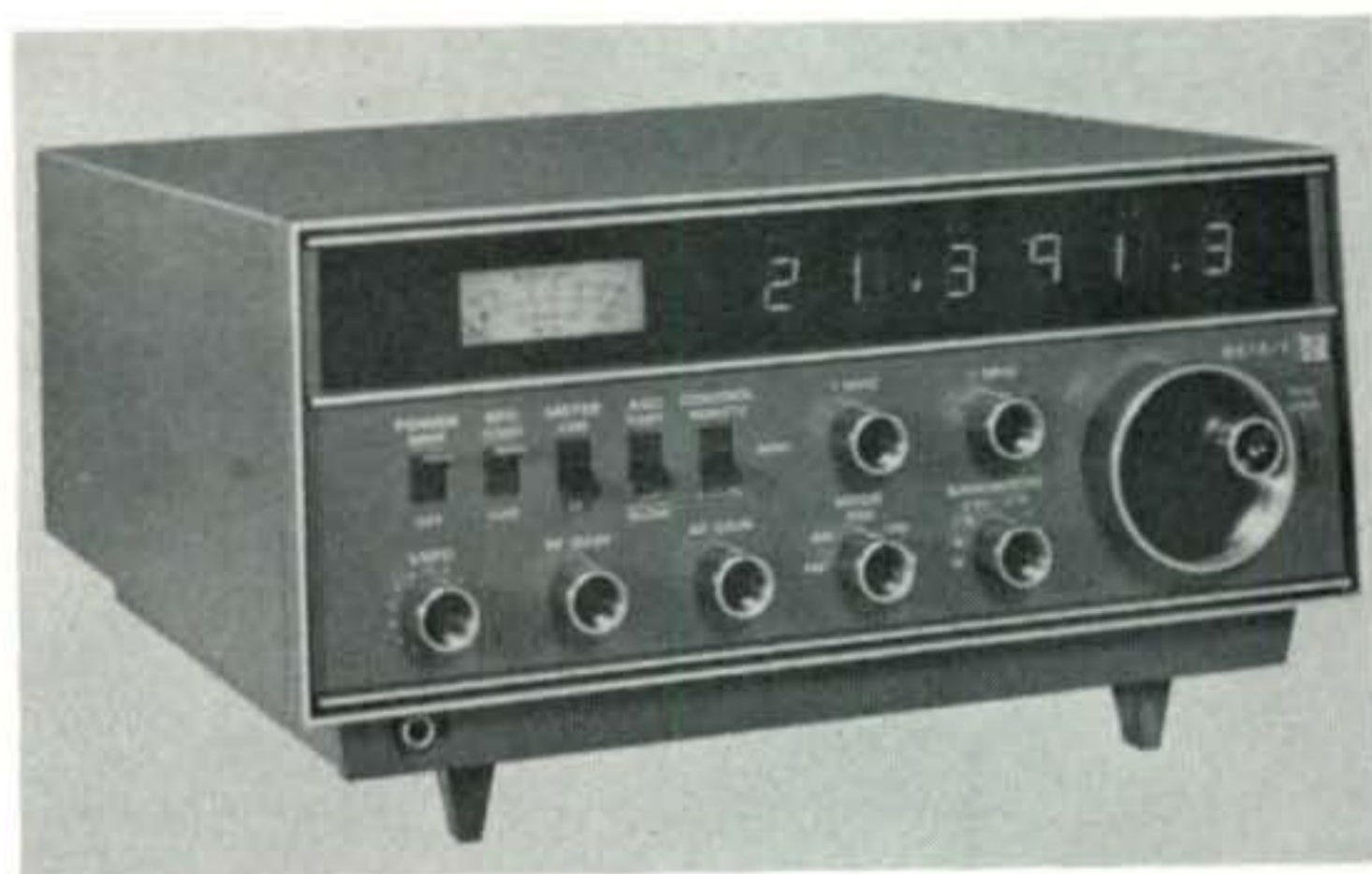
The newer Collins 651S-1 general purpose h.f. receiver.
